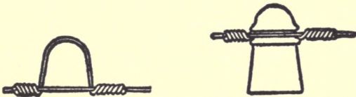
Transmission wire on glass insulator
