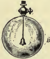
FIG. 2.—TRANSMISSION OF SOUND THROUGH A VACUUM.
