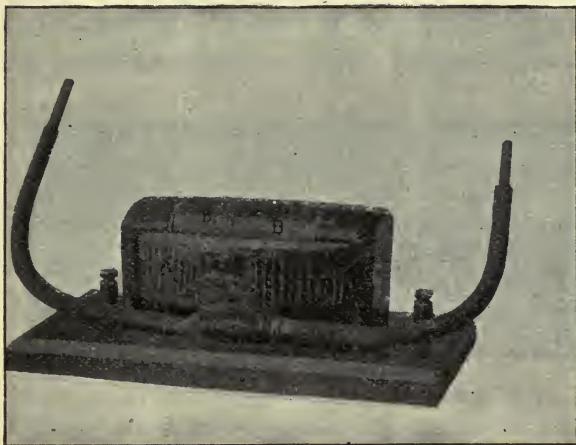
FIG. 78.—ALTERNATING-CURRENT TRANSFORMER, FERRIC MAGNETIC CIRCUIT.
