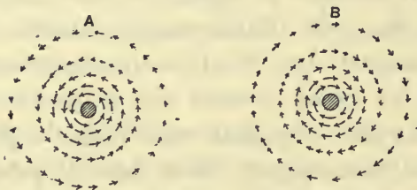
FIG. 75.—MAGNETIC FLUX PATHS SURROUNDING A STRAIGHT ACTIVE CONDUCTOR.
