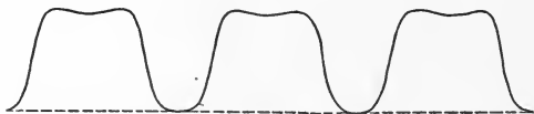
FIG. 92.—DIAGRAM OF A POSSIBLE WAVE FORM OF MAGNETO-ELECTRIC GENERATOR E. M. F. (WHEN A COMMUTATOR IS EMPLOYED).
