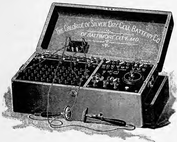
FIG. 108.—INDUCTION COIL WITH BATTERY OF CHLORIDE OF SILVER CELLS.
