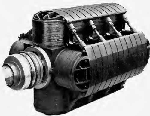
PLATE 8C.—Revolving Field Magnets of Three Phase Alternator for Direct Driving from a Steam Turbine, made by Messrs. Dick, Kerr & Co. The Rings shown on the Axle are to deliver the Current to the Field Coils.
