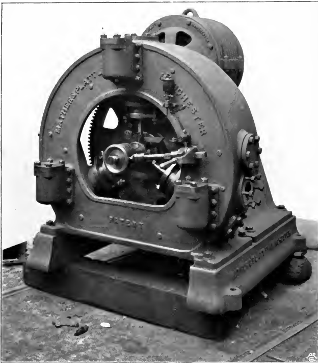
PLATE 23B.—Mather & Platt's Variable Stroke Three Throw Ram Pump, driven by an Electric Motor. The three Cylinders are arranged round the Containing Cylinder, and the Stroke is regulated by the Lever on the Right.
