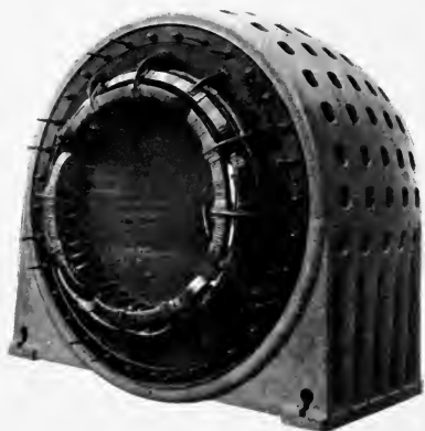
PLATE 8B.—Armature of Three Phase Generator for Turbo Driving, with Coils complete, made by Dick, Kerr & Co.
