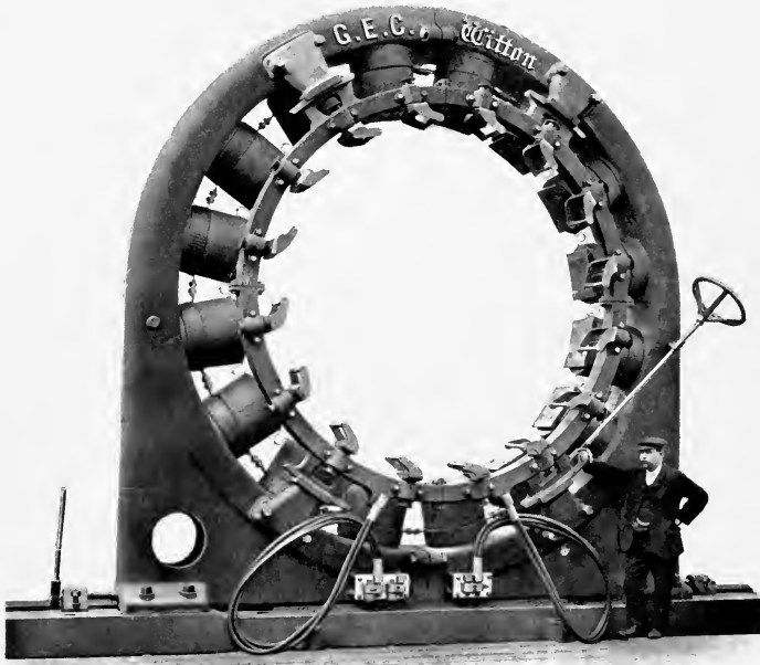
PLATE 7A.—Enclosing Ring, Field Magnet Coils, Pole Pieces, and Brush Gear of a Multipolar Continuous Current Generator, by the General Electric Co.
