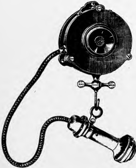
FIG. 20.—Simple Telephonic Apparatus for Use in Mines, consisting of Microphone Transmitter, Telephone Receiver, and Switch, the Telephone Cord and the Receiver being protected by a wrapping of Brass Tubes.
