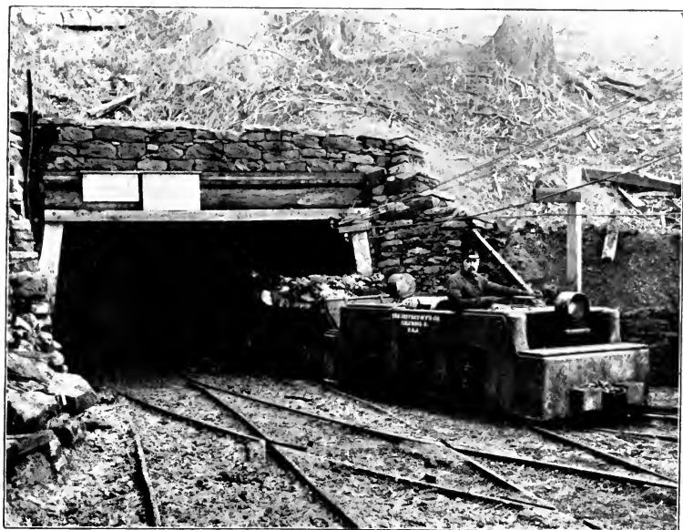
PLATE 26B.—Electric Mine Loco, as employed in America and on the Continent, made by the Jeffrey Co.
