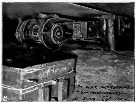
PLATE 31D.—Blackett's Underground Coal Conveyor, for use at the Face of the Coal, driven by a Continuous Current Motor. The Coal is seen coming out on the Conveyor and tipping into the Tub at the End of the Road.
