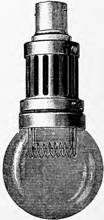
Fig. 50.—"B" Form of Nernst Lamp with Horizontal "Glower" and Heating-coil and Globe. The Holder, with the Electro-magnetic Cutout and Resistance, are inside the Metal Case forming the Upper Part of the Apparatus.
