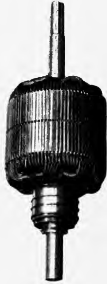
PLATE 19D.—Wound Rotor of Three Phase Motor with Slip Rings for connecting to Starting Resistance. [To face p. 272.]
