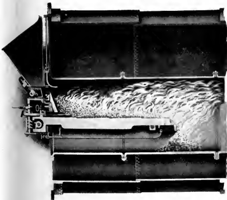
PLATE 2C.—Longitudinal Section of Lancashire Boiler fitted with Hodgkinson's Mechanical Stoker. The Hopper and Gear are seen on the Left.
