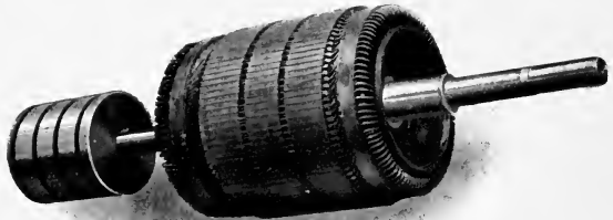
PLATE 22C.—Wound Rotor of Two Phase Motor, with Rings for connecting to Starting Resistance.
