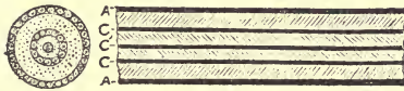
FIG. 188.—Sectional View of Nolet Safety Cable. A, Armouring; C, Main Cable; C 1 , Auxiliary Conductor.
