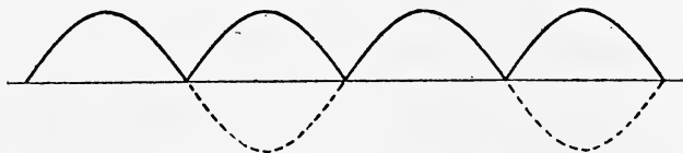
FIG. 176.—Rectified Alternate Current.
