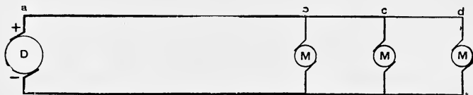
FIG. 58.—Simple Parallel System.
