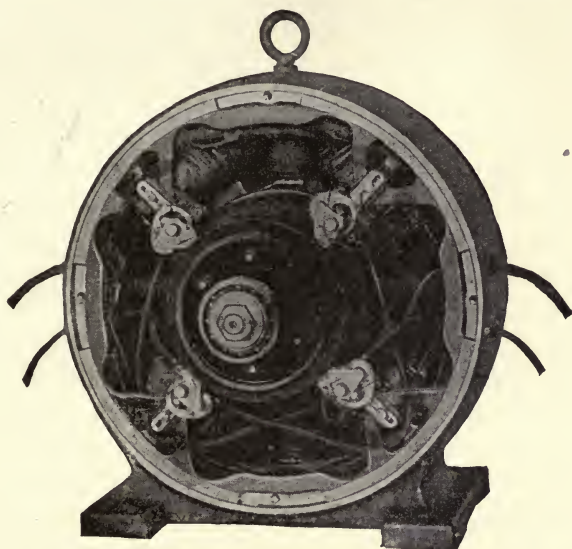
FIG. 21. — INTERPOLAR MOTOR — FRONT BEARING REMOVED.
