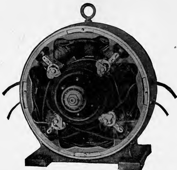
FIG. 21. — INTERPOLAR MOTOR — FRONT BEARING REMOVED.
