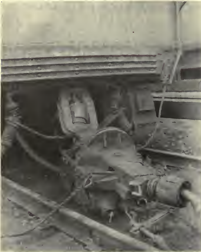
The cars became coupled at the time of the collision, but the impact broke the coupler support of the colliding car. As the stationary car went forward from the blow, it took both couplers with it, as shown in the left-hand view. The right-hand view shows the end of the colliding car with the damage done to the anti-climber. Except for broken glass, there was practically no other injury to the cars
