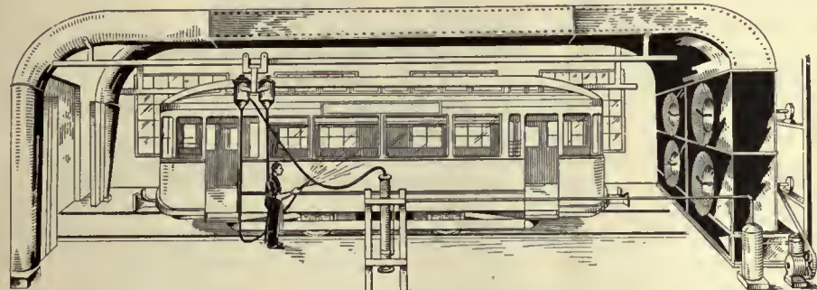
Room for spray painting arranged with horizontal air flow. Convenient connections for compressed air are installed
