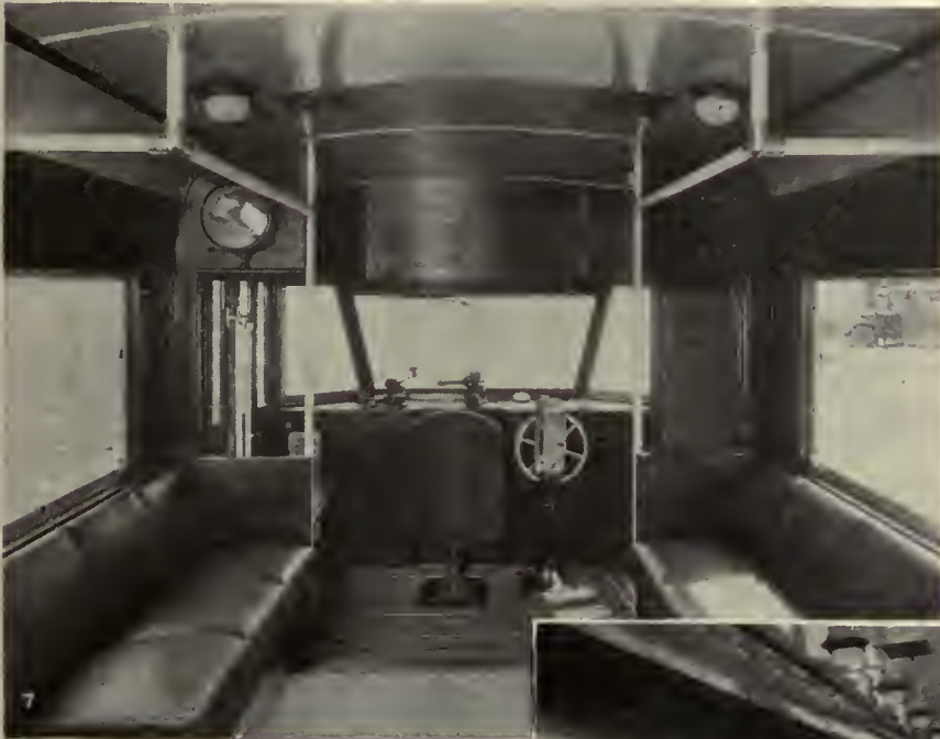
All control apparatus is within easy reach of the seated operator in this compactly arranged vestibule
