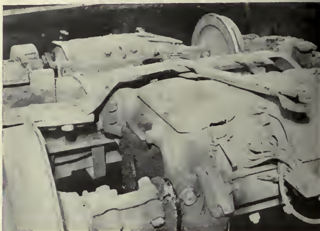
A 40-hp. railway motor as it was received in the shop after one year's operation in city service
