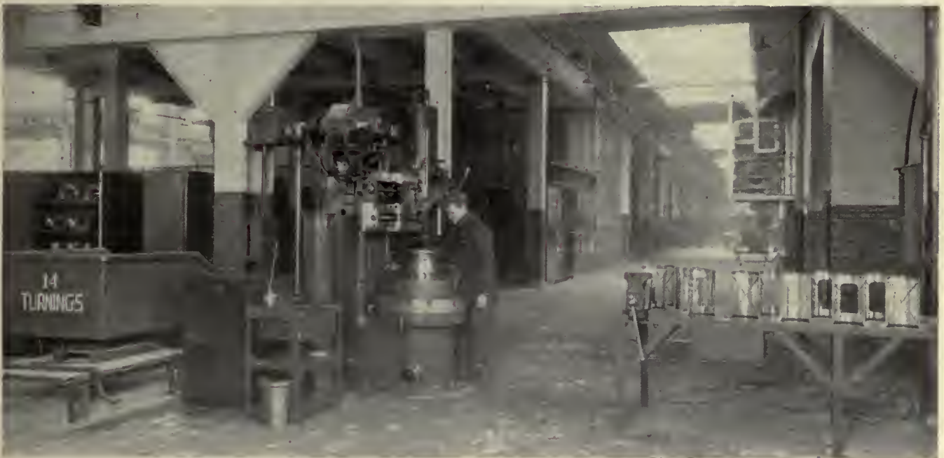
The two halves of axle bearings are bored out at one operation in a vertical boring mill
