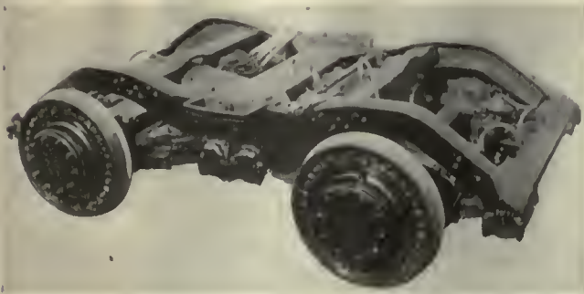
The Timken worm drive trucks used under one of the Pittsburgh cars are equipped with 35-hp. motors and automotive type spring mounting
