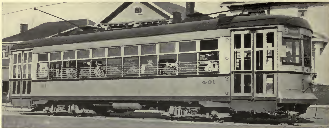
Twenty double-truck cars of this type were completely renovated and equipped for one-man operation. Automatic rear-exit treadles have since been installed on twelve of them
