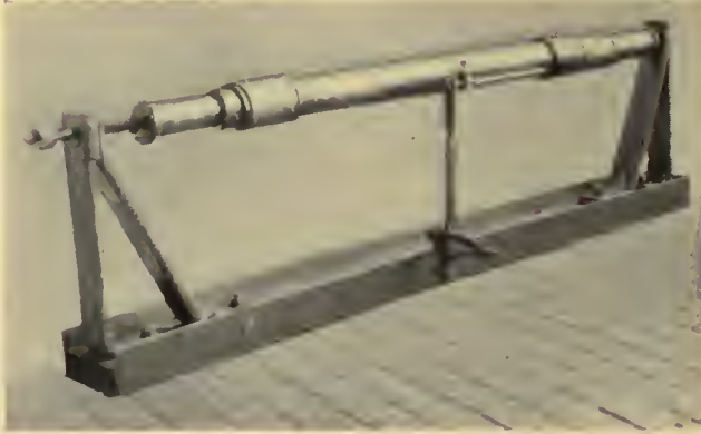
Testing an axle for eccentricity by means of a jig made in the Norfolk shop of the Virginia Electric & Power Company
