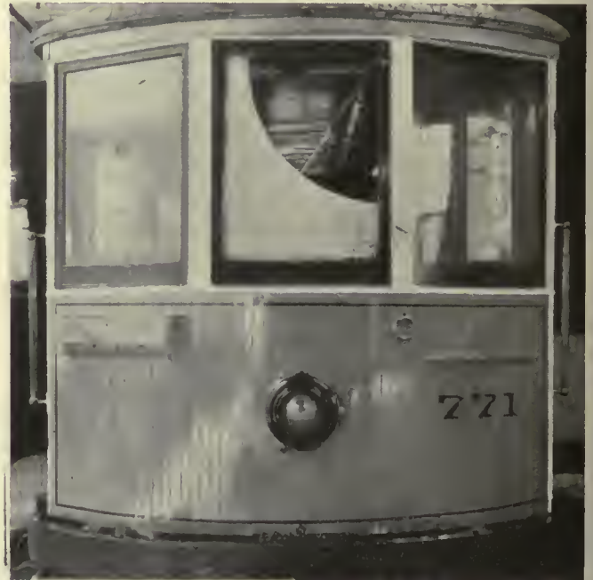
Window wipers on cars of the Connecticut Company clear a large area of the glass in front of the motorman
