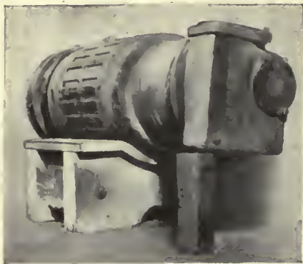
Armatures are kept off the floor with this type of stand
