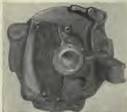
Correctly packed pinion end housing for oil and waste lubrication showing wool waste in place
