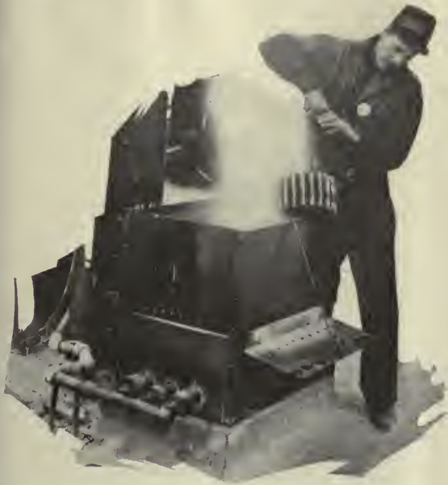
Removing a pinion from the hot water tank for installation on armature shaft
