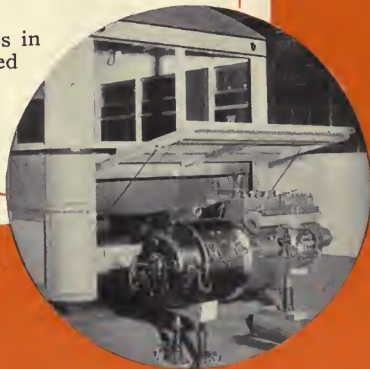
Showing engine installed and manner in which panel lifts up for inspection or removal.
