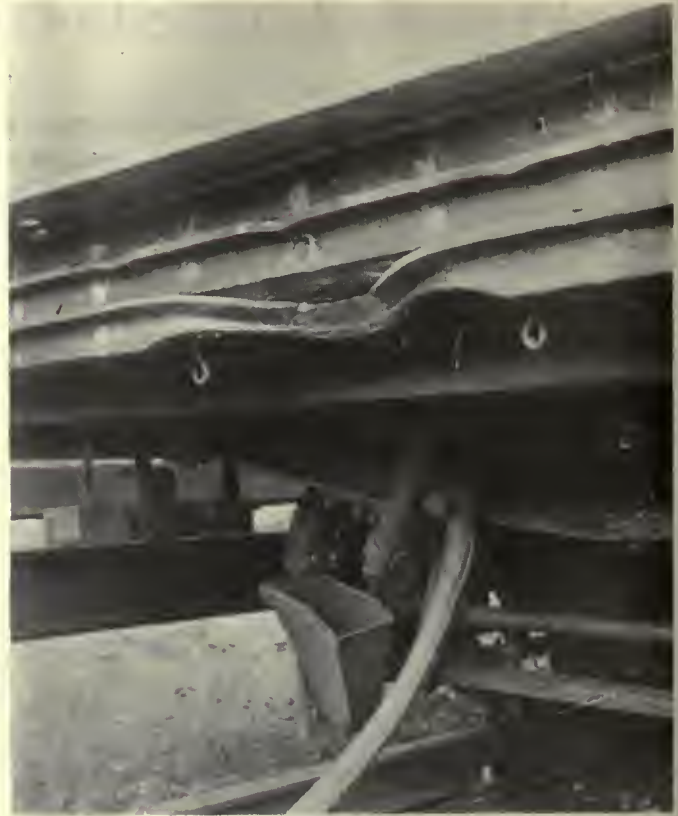
The cars became coupled at the time of the collision, but the impact broke the coupler support of the colliding car. As the stationary car went forward from the blow, it took both couplers with it, as shown in the left-hand view. The right-hand view shows the end of the colliding car with the damage done to the anti-climber. Except for broken glass, there was practically no other injury to the cars
