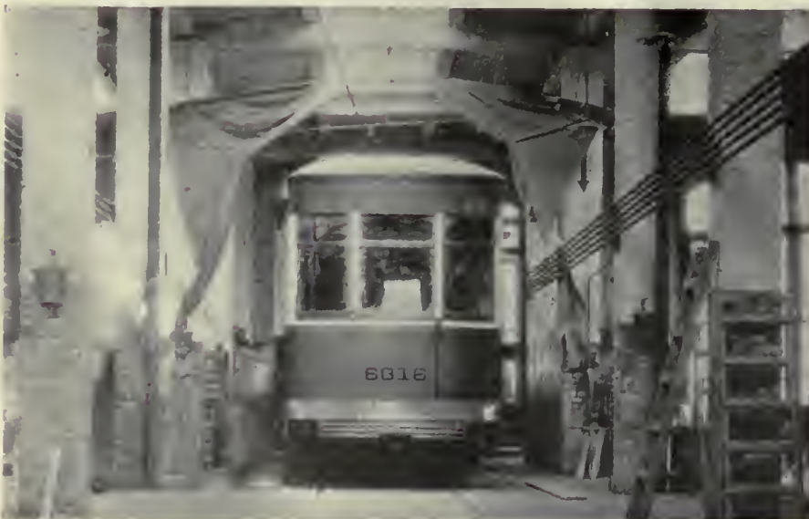
At left—After three coats of flat color have been applied and lettering and striping done, the car is given three coats of varnish. At right—Lettering and striping are done by hand
