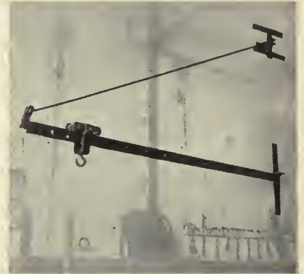
These booms were not expensive to construct and have been satisfactory for truck overhauling
