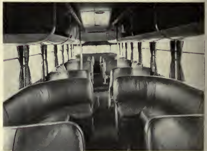
Seats over the wheel housings in this Twin Coach are a departure from the ordinary type
