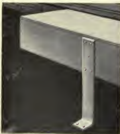
Additional support installed on sand hopper
