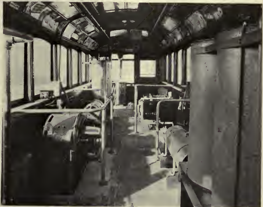
Interior arrangement of grinder car
