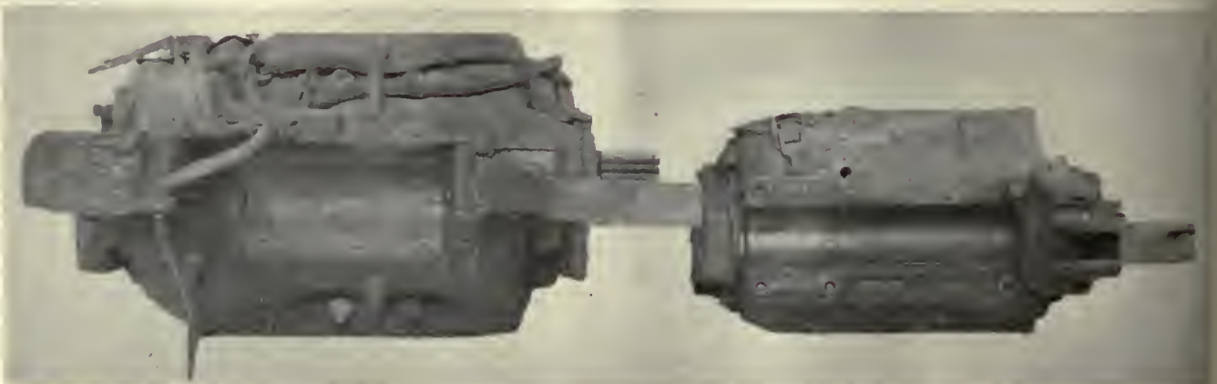
The old type motor at the left weighs 2,880 lb., while the new one at the right, a light-weight motor adopted as standard by the Georgia Power Company, weighs 1,415 lb.
