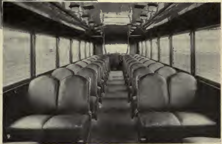
Leather-upholstered, deep spring-cushioned seats insure passenger comfort. The car is arranged for double-end operation. Note the overhead rail handholds in the corners of the body
