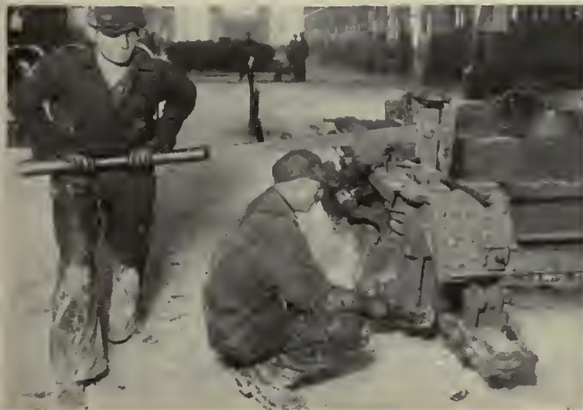
Bolts are installed under journal boxes quickly by means of a lever attachment that compresses the spring between the truck frame and the top of the journal box
