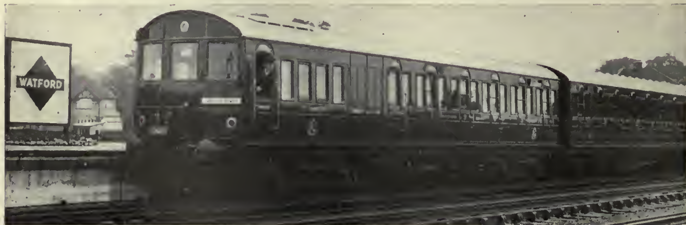
The new seven-car subway train for the Metropolitan Railway of London carries 482 passengers seated and has a starting effort of more than 30,000 lb.
