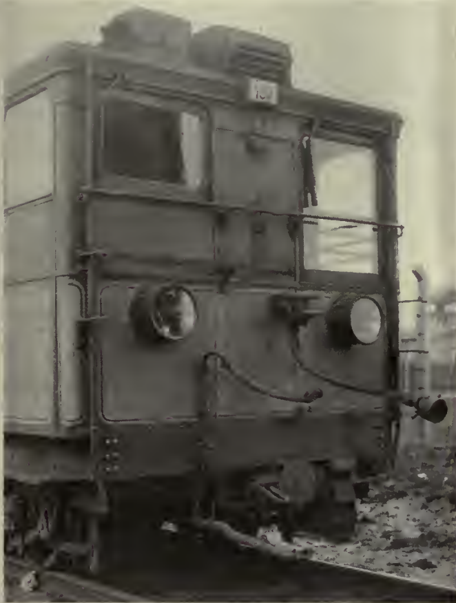
At left, end of Hamburg elevated car before addition of automatic coupling and anti-climber. At right, after their addition
