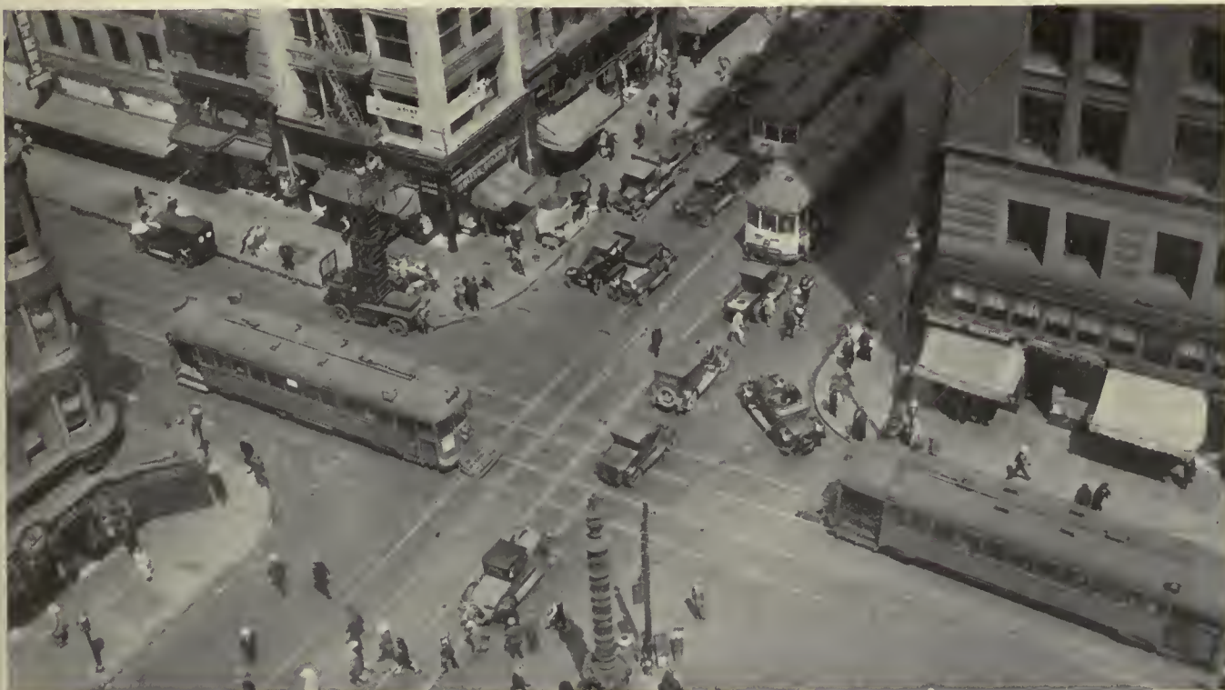
Far side car stops on the north side of Market Street cause congestion, in the opinion of the authors of the report
