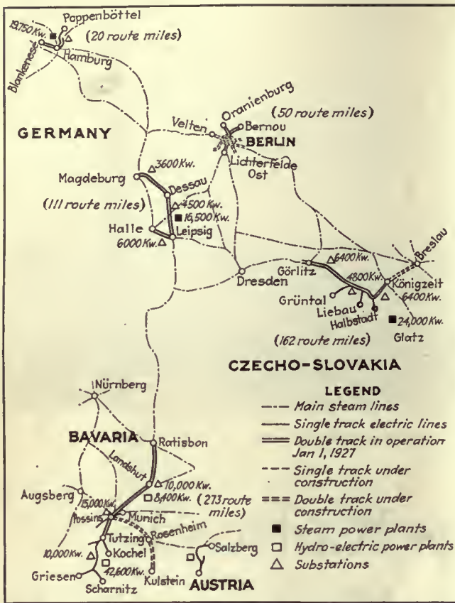
Five principal regions are served by the electrified lines of the German Federal Railroad Company
