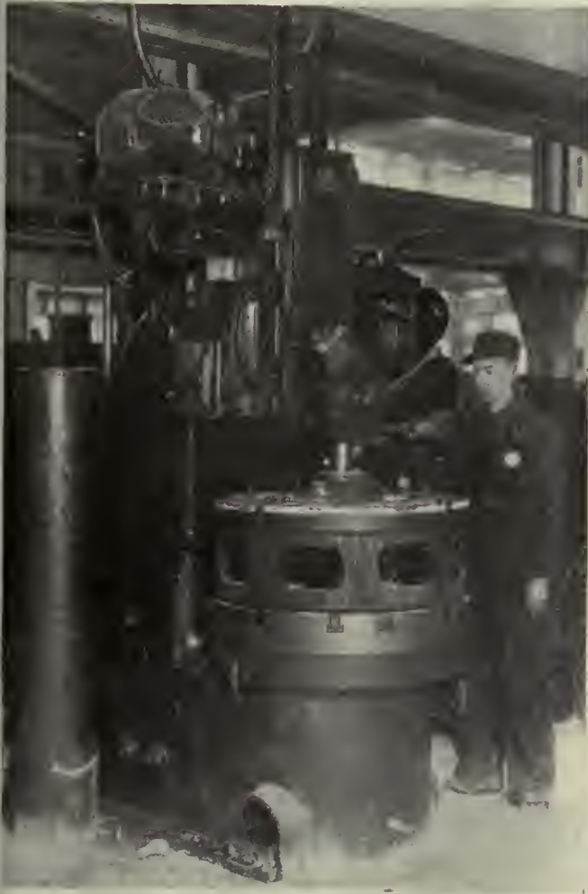
Boring out an armature bearing after it has been pressed into housing. A special jig is used for centering the housing accurately
