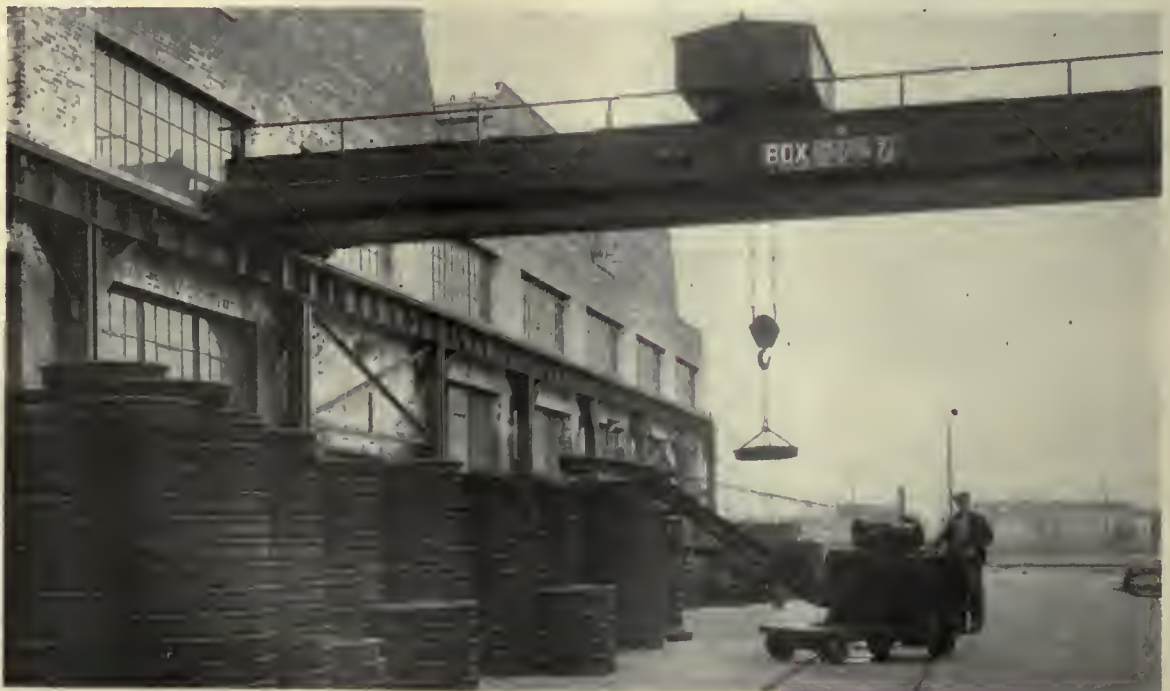
A convenient departmental storage for wheels and axles speeds up production. Material can be brought in on a car and unloaded by the overhead 7½-ton traveling crane. Wheels are loaded on small trucks and taken to the wheel and axle department by electric crane trucks
