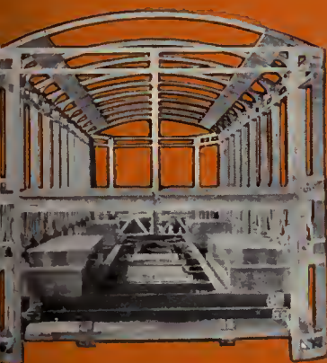
Rear view of Versare frame showing engine mounting and heavy channels affording protection at corners. When engine is installed this channelling extends clear across the back behind the bumper.
