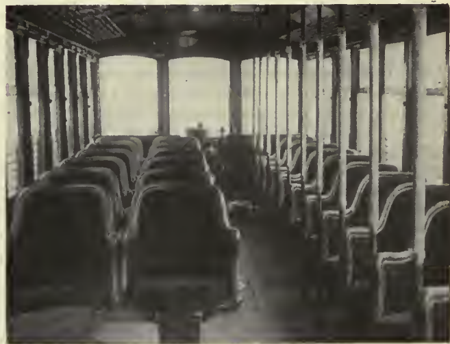
Seats in the parlor compartment are upholstered in green plush, with leather arm rests, as shown. The seats in the smoking compartment are upholstered in green leather
