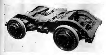
The Timken worm drive trucks used under one of the Pittsburgh cars are equipped with 35-hp, motors and automotive type spring mounting
