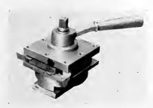
Four-way tool-post holder for use on lathe
