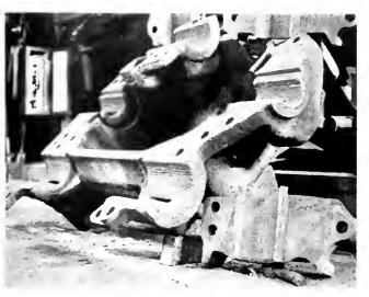
GE-80 bearing fits welded and ready for machining
