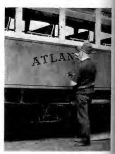
At left—After three coats of flat color have been applied and lettering and striping done, the car is given three coats of varnish.
