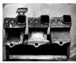
Three stages in changing the waste window of GE-80 axle con left. Center, ¼-in. plate installed and ready for weldin Right, welding completed.
