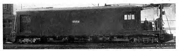
Snow plows have been attached to a motor work car for use on the Dorchester rapid transit extension
