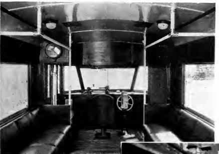
All control apparatus is within easy reach of the seated operator in this compactly arranged vestibule
