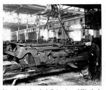
Stirrups fit over the ends of elliptic springs and lifting by the crane compresses them so that they fall into position readily
