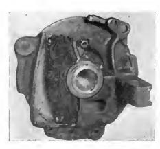
Correctly packed pinion end housing for oil and waste lubrication showing wool waste in place
