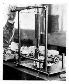
Testing brush-holder spring tension by a special device in the shops of the Brooklyn-Manhattan Transit Lines
