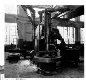
At top—Boring out a subway wheel. The wheel suspended from the crane on the left is ready to be swung into position. A truck at the right receives wheels after they are bored. The crane at the right handles finished wheels
