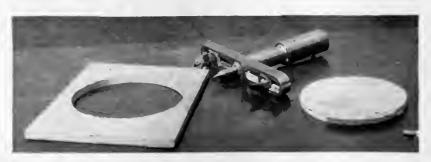
Convenient tool for cutting holes in dust guards
