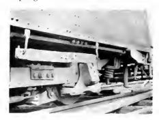
Car numbers are welded on the drawbars
