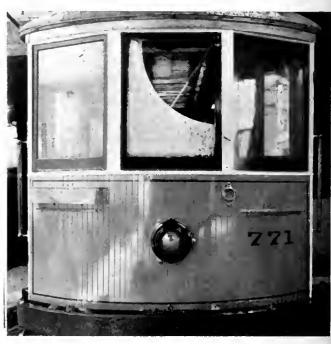
Window wipers on cars of the Connecticut Company clear a large area of the glass in front of the motorman
