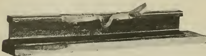
Copper-Welded Rail Bonds—Clay Mold Removed Showing Extra Copper Ready for Trimming.
