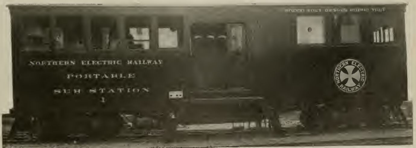
Northern Electric Railway—Portable Substation with 60,000-Volt Transformers and Motor-Generator Set.
