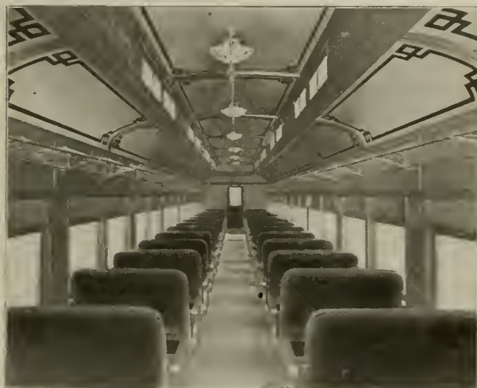
Indestructible Fiber—Interior of Long Island Railroad Coach with Indestructible Fiber Headlining.
