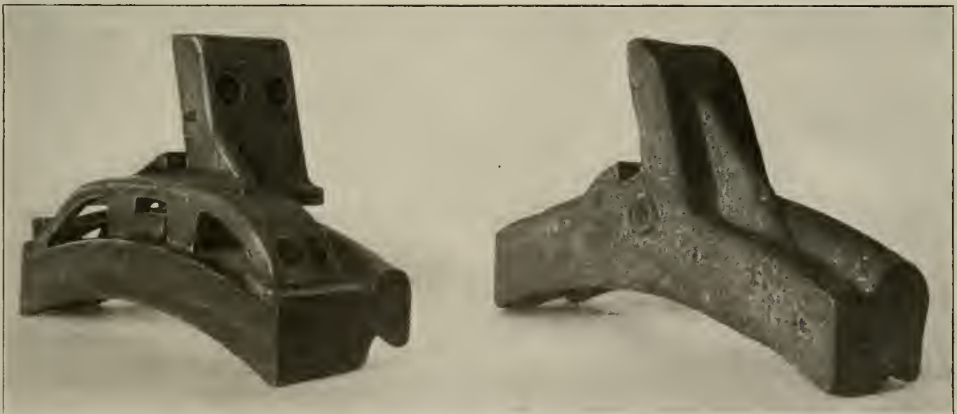
Standardizing Brakeshoes—Present Practice Shown at the Right, with Flanged Shoe and Attachment Conforming to Recommendation at the Left.
