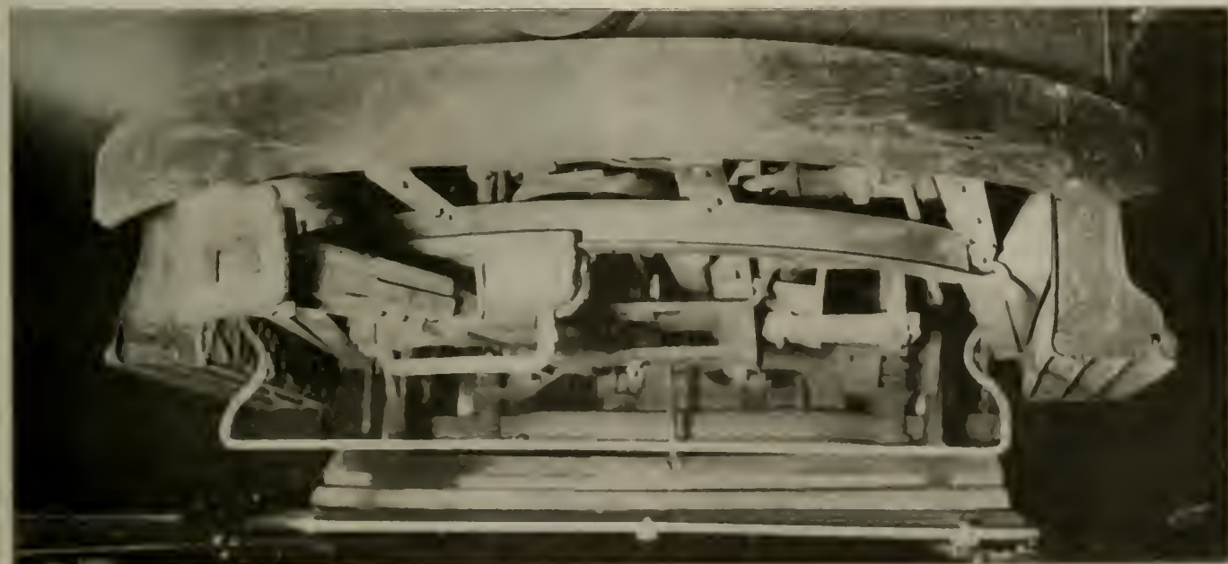
Shop Practice at Memphis—Front of Car Showing Radial Draft Rigging and Automatic Drop Fender.
