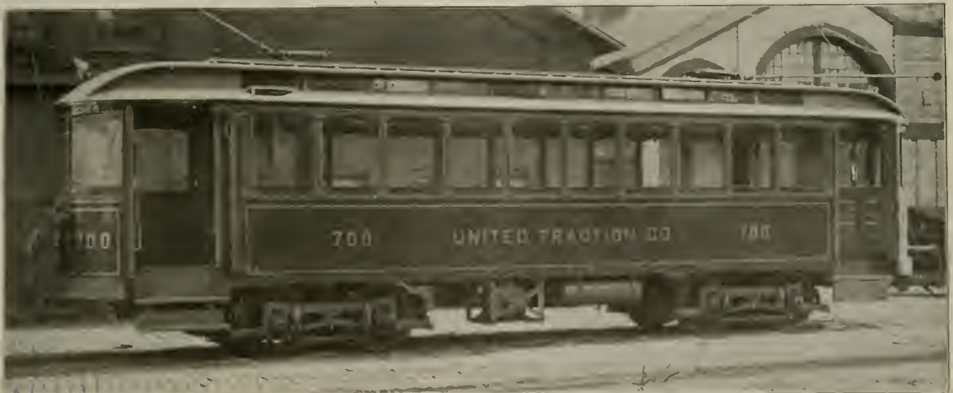
New Cars for United Traction Company, Albany—Exterior View showing Air-Operated doors and steps.
