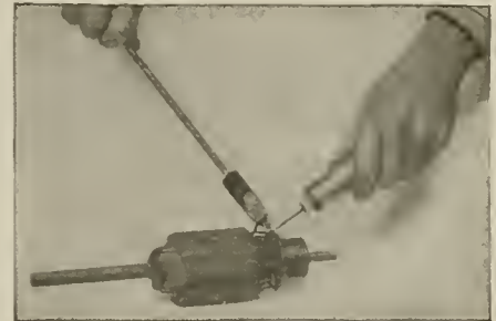
Blake Tube Flux—Method of Application.
