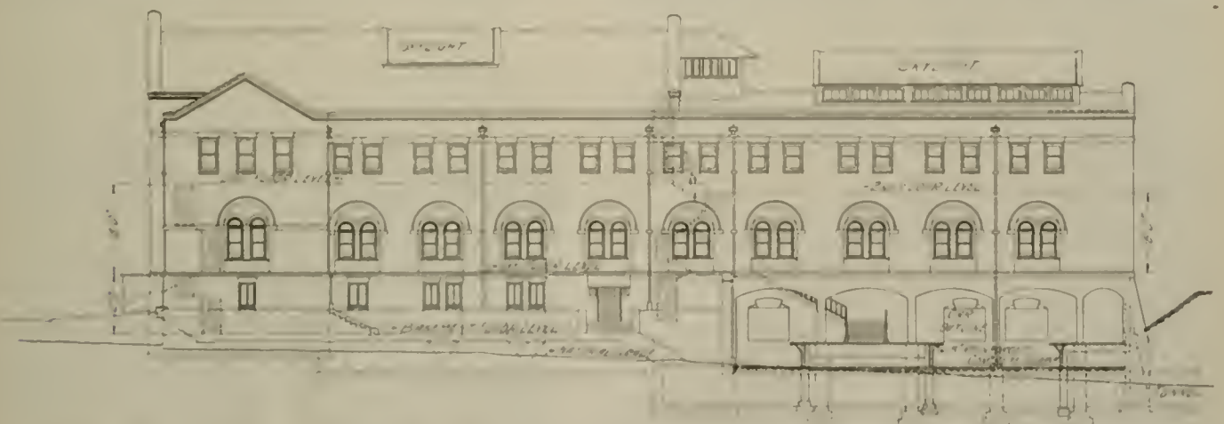
Market Street Terminal, Philadelphia—East Elevation Showing Platform Arrangement for Philadelphia Rapid Transit Trains.
