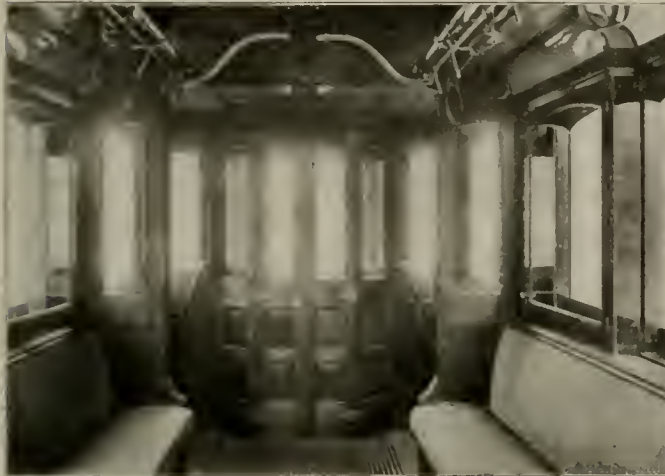
New Cars for United Traction Company, Albany—Interior View Showing Arrangement of Doors to Form Motorman's Compartment.
