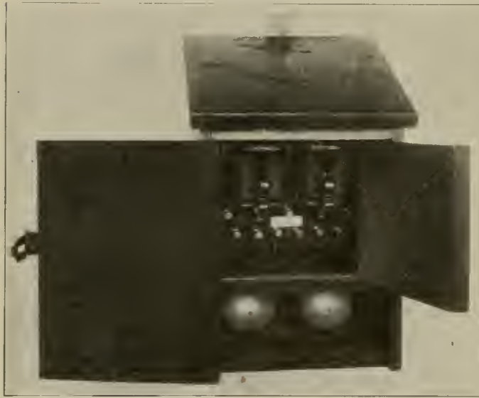
National Crossing Signal—Relay and Case as Mounted Near Contact Maker.
