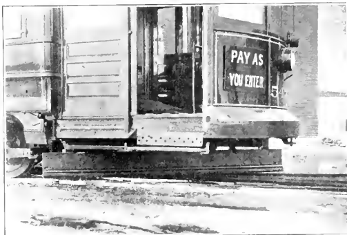
Chicago City Railway—Front of Car, Showing New Life Guard.
