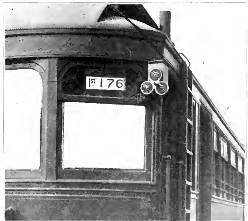
Gibbs Train-Indicating Device—View as Installed in Car.
