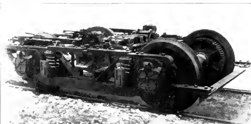
New Elevated Cars for Brooklyn Rapid Transit Company—Side View of Motor Truck.
