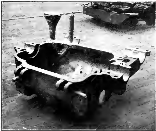
Chicago City Railway—Motor Shell with Thermit Repair.
