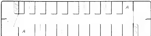
Long Single-Truck Cars Without Monitors—Floor Plan of Car No. 14, Showing Arrangement of Vestibule Doors.
