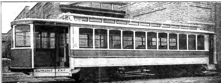
Type "Pay-as-you-enter" Cars. 200 Built for The Public Service Railway Company, New Jersey
