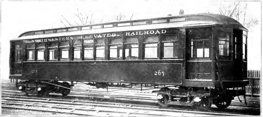
Northwestern Elevated Cars—Side View, Showing Large Air Operated Doors.
