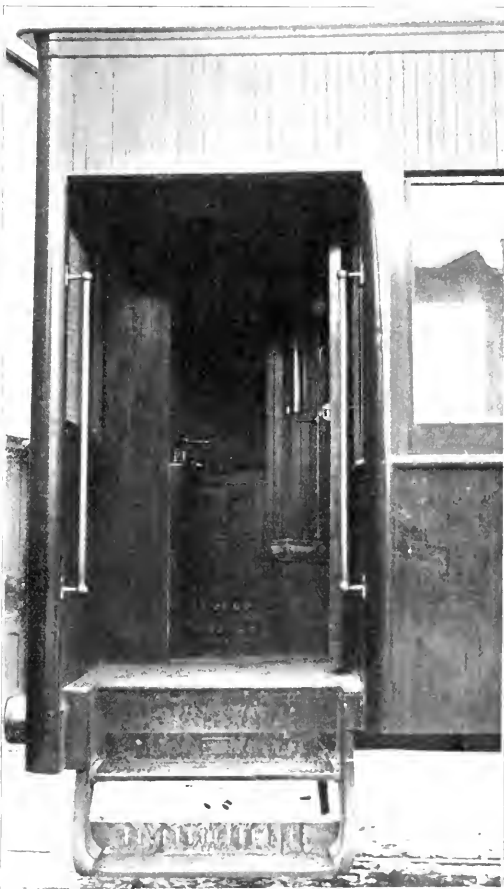
Long Single-Truck Cars Without Monitors—Front Platform of Car No. 14, Showing Motorman's Compartment.
