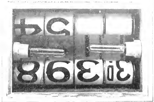
Gibbs Train-Indicating Device—Rear View with Cover Raised.
