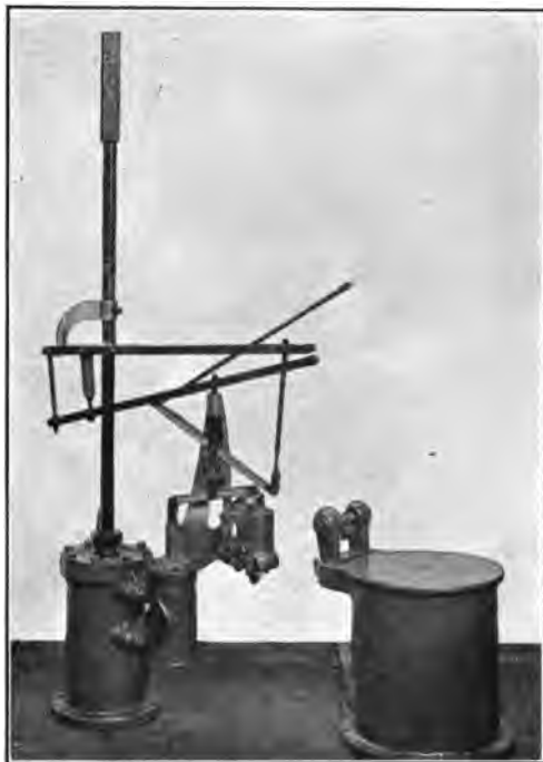
FIG. 81.—U. S. S. California : Hydraulic Operating Mechanism and Operating Governor for Propulsion Unit No. 1
