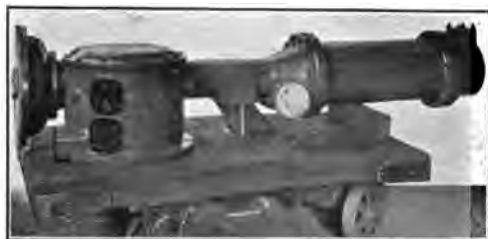
FIG. 82.—U. S. S. California : Spiral Gear Driven Oil Pump for Propulsion Unit No. 1
