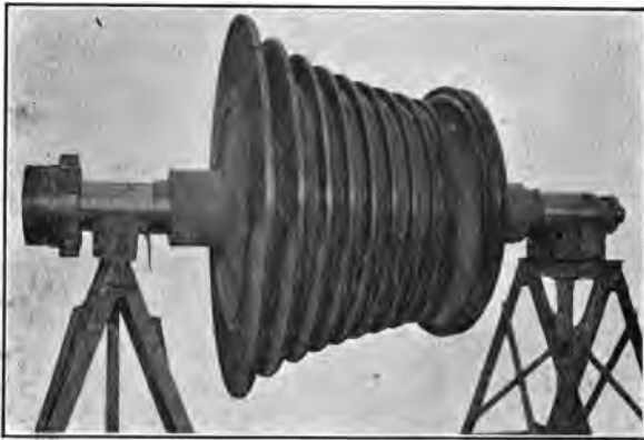
FIG. 80.—U. S. California : View of Assembled Turbine Rotor for Propulsion Unit No. 1.
