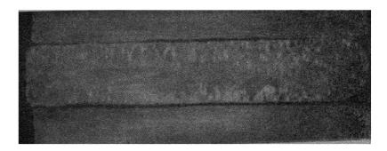
Fig. 120. Poor penetration at both edges.
