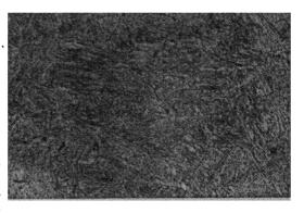
Fig. 201. Micrograph of electric slag weld made in steel 25 × 3H M after hardening and tempering (magnification × 300).
