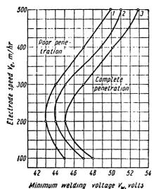
Fig. 39. Ratio of least welding voltage to welding speed giving full penetration and fusion at various thicknesses per electrode:
