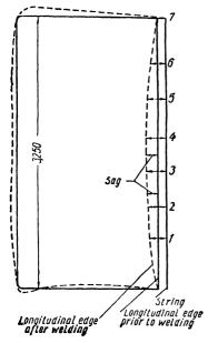
Fig. 133. A shell course of a high-pressure boiler before (straight line) and after (dotted line) electric slag welding of one longitudinal seam.
