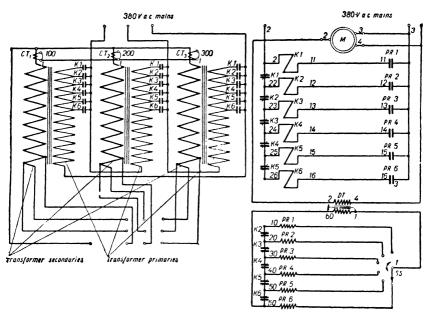
Fig. 169. Schematic diagram of the TIIIC-1000-3 welding transformer.
