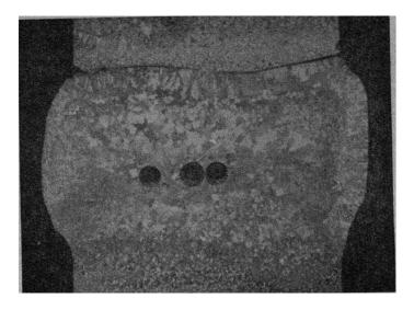
Fig. 206. (ras pockets in electric slag weld made with damp flux; poor fusion can be seen on one side.
