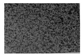
Fig. 182. Micrograph of a welded joint in Grade 40 steel after normalising (fusion area) (magnification × 60).
