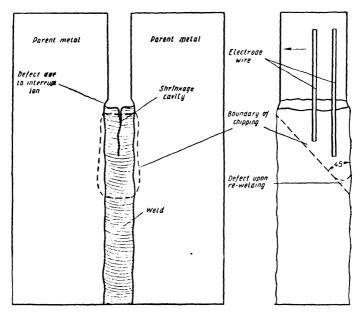
Ftg. 222. Deseaming a weld after inadvertent stoppage of electric slag welding.
