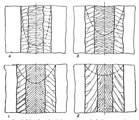
Fig. 45. Effect of metal pool shape on the growth of columnar crystals:
