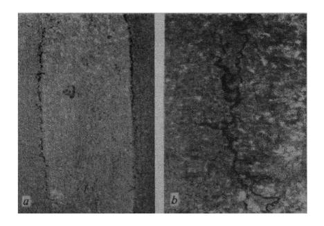
Fig. 116. Cracks in the near weld zone. a-magnification > 1, b-magnification > 8
