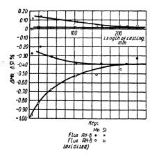
Fig. 59. Variations in recovery of manganese and silicon with length of ingots welded with AH-8 flux and  $CB-10\Gamma2$  wire.
