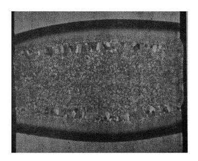
Fig. 199. Macrograph of a word joint in Cr-Ni-Mo steel after welding.
