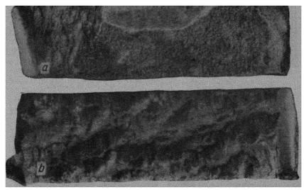
Fig. 114. Weld fractured along crack:
