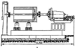
Fig. 165. Welding unit: e-for shafts of hydraulic turbines; b-for cylinders of power presses (diagram).
