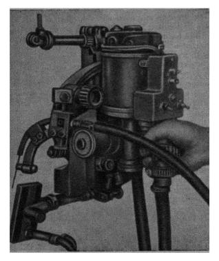
Fig. 150. Type A-501 was a magnet automatic weider (general view).
