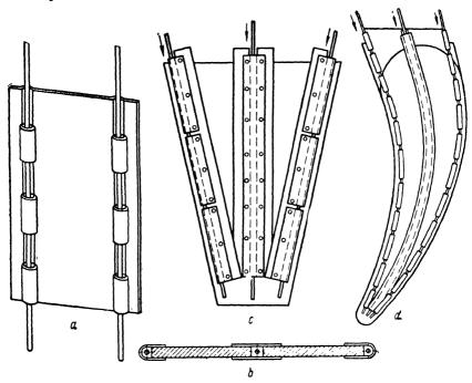
Fig. 97. Designs of consumable electrode guides.
