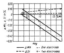
Fig. 62. Recovery of manganese and silicon from AH-8 flux by deposited metal as a function of manganese content in electrode wire.
