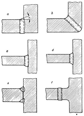
Fig. 82. Types of corner joints.
