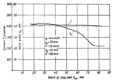
Fig. 32. Welding current and were width plotted against depth of slag pool.
