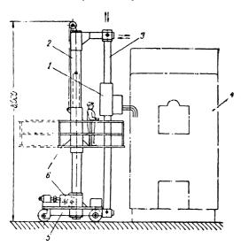
Fig 162. Tower-type universal unit incorporating an A-372P welding apparatus: 1—welding apparatus; 2—load-bearing tower; 3—rail track for welding apparatus; 4—workpiece; 5—truck, 6—lift for operator's cab; 7—lifting and ro-
