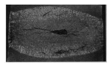
Fig. 115. Cracks and shrinkage cavity at the end of a weld.
