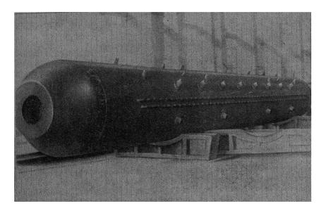
Fig. 218. Drum for Type TII-230 boiler
