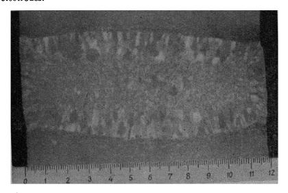
Fig. 185. Macrostructure of a welded joint in steel 40 made with two C<sub>B</sub>-10Γ2 wire electrodes at a welding speed of 370 m/hr.
