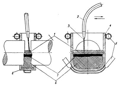
Fig. 257. Semi-automatic electric slag welding of reinforcing bars:
