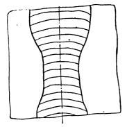
Fig. 128. Variations in the width of a weld near the surface of plates.
