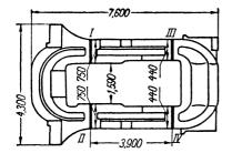
Fig. 238. Sketch of a rolling mill stand; IV-I—butt welds.
