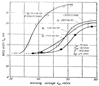
Fig. 28. Weld width plotted against welding voltage.
