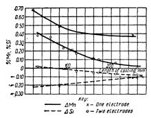
Fig. 58. Variations in recovery of manganese and silicon with length of ingots welded with AH-8 flux and one or two CB-10ΓC wire electrodes.
