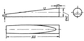
Fig. 88. Cylindrical wedge employed in fitting up jobs for electric slag welding.
