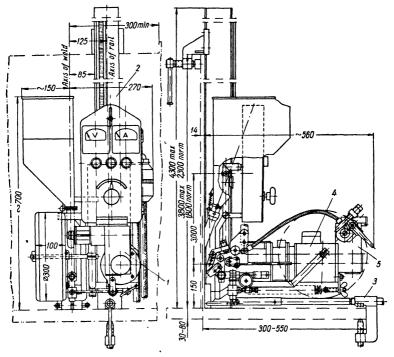
Fig. 136. Type A-314 single-motor rack-riding welding apparatus.
