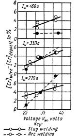
Fig. 66. Oxidation of chromium in submerged arc and electric slag hard-facing.
