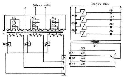
Fig. 170. Schematic diagram of the TIIIC-3000-3 welding transformer.
