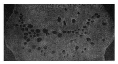
Fig. 118. Gas pockets in the weld metal.
