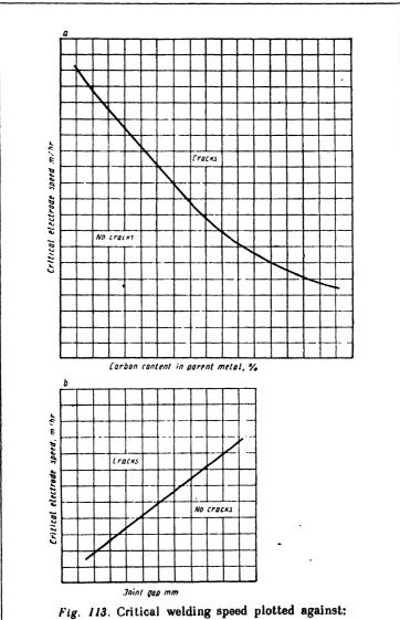
Fig. 113. Critical welding speed plotted against:
