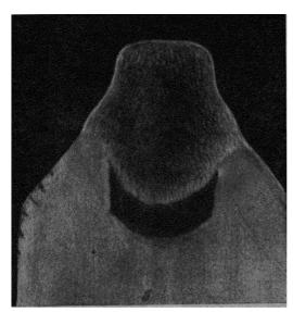
Fig. 214. Macrograph of tong bit hard-faced with steel 3\(\chi 2B8\).
