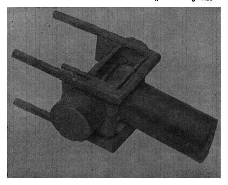
Fig. 256. Water-cooled mould for the electric slag welding of reinforcing bars.
