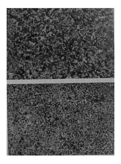
a plate electrode of the same material (magnification  $\times$ 60): weld after normalising; d—open-grain area after normalising.
