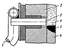
Fig. 175. Horizontal copper prod: 1-cooling water; 2-moulding shoe; 3-copper prod; 4-slag pool; 6-metal pool; 6-weld
