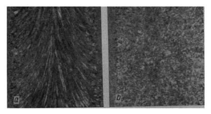
Fig. 52. Macrostructure of Type IV weld: a—section along weld; b—section across weld.
