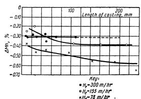
Fig. 71. Oxidation of manganese plotted against welding speed.
