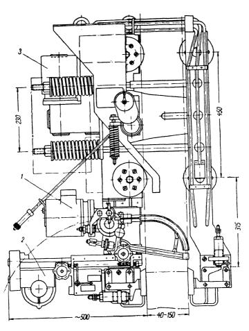
Fig. 147. Type A-340 single-electrode trackless automatic welder.
