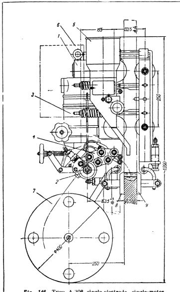
· Fig. 146. Type A-306 single-electrode single-motor trackless automatic welder.
