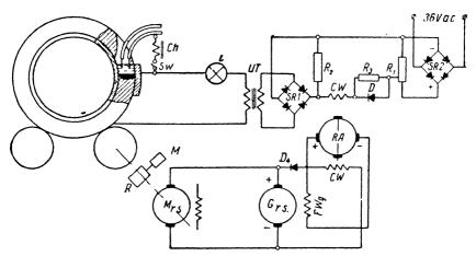
Fig. 177. Schematic diagram of weld-pool level control on circumferential seams.
