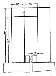
Fig. 90 End clamp and finishing tabs.
