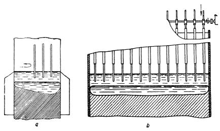
Fig. 7. Diagram of electric slag welding on heavy sections:
