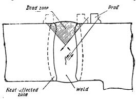
Fig. 130. Diagram of ultrasonic quality inspection of a butt weld.
