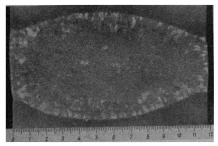
Fig. 180. Macrostructure of a welded joint in steel 40.
