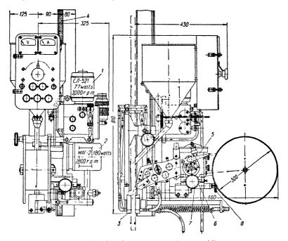
Fig. 137. Type A-433 double-motor rack-riding welding apparatus.
