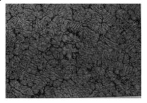
Fig. 215. Micrograph of P-18 deposited metal (magnification ×100).
