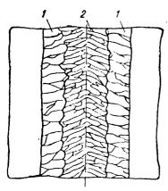
Fig. 44. Schematic structure of Type I weld.
