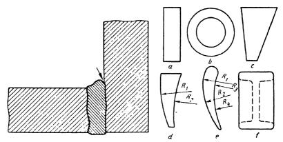
Fig. 83. Overlapping in poorly designed corner joint.
