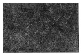
Fig. 202. Micrograph of superheated area in near-weld zone in steel 25X3HM after hard-ening and tempering (magnification ×300).
