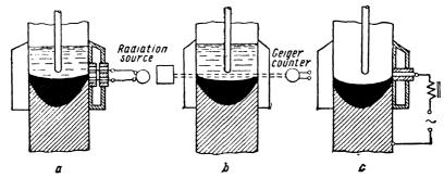
Fig. 173. Level gauging in the metal pool.
