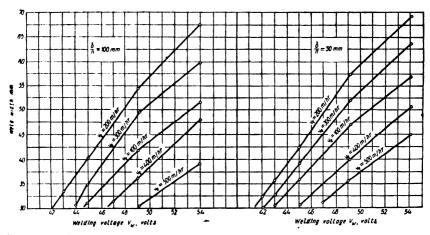
Fig. 29. Weld width plotted against welding voltage at various welding speeds.
