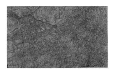
Fig. 196. Microsection of near-weld zone with tears.
