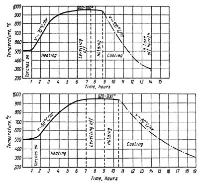
Fig. 230. Heat treatment of TΠ-230 boiler drum welded by the electric slag process:
