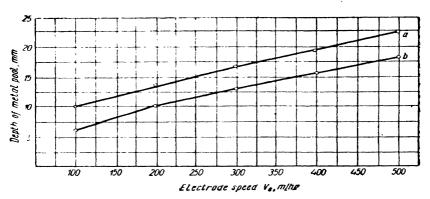
Fig. 27. Depth of metal pool plotted against welding speed at various values of  $\frac{\delta}{n}$ :
