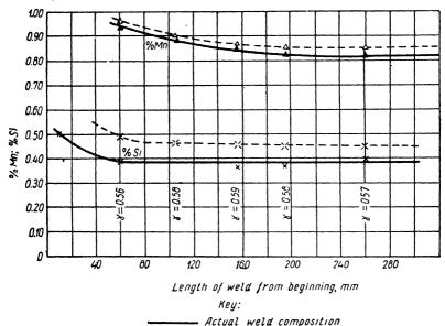
Fig. 65. Comparison of actual and design contents of impurities in weld metal in electric slag welding with CB-10ΓC wire.
