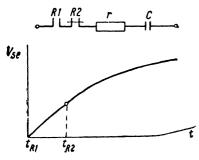
Fig. 178. R-C circuit for measuring the depth of the slag pool.
