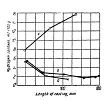
Fig. 77. Variations in hydrogen content in ingots of steel X25H20 cast by electric slag process with a.c.:
