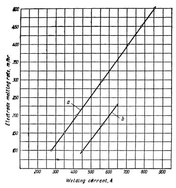
Fig. 18. Speed of wire feed plotted against welding current in submerged arc and electric slag welding:
