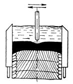
Fig. 40. Schematic diagram of metal pool in welding with one moving electrode.
