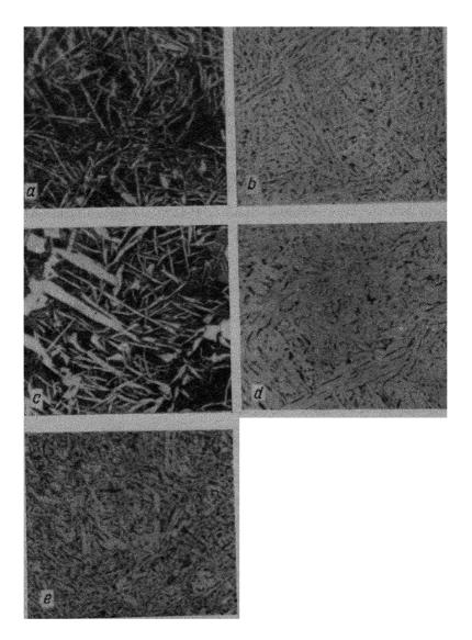
Fig. 55. Secondary structure of weld metal (magnification $\times$ 150): a—coarse columnar grains in Type I and II weld; b—coarse columnar grains in Type II and II welds; d—fine columnar grains in Type I and II welds; d—fine columnar grains in Type IV weld; e—equi-axial grains.
