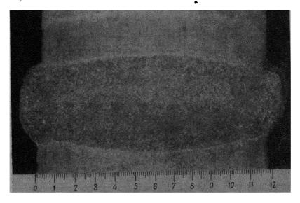
Fig. 186. Macrostructure of a welded joint in steel 40 made with a plate electrode of the same material
