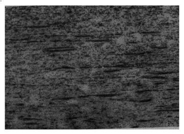
Fig. 231. Baumann replica of steel 22K plate 250 mm thick in the area corresponding to the head of an ingot.
