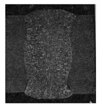
Fig. 37. Electric slag weld obtained without weaving motion of electrodes.
