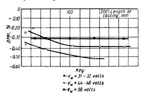
Fig. 73. Oxidation of manganese plotted against welding voltage.
