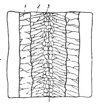
Fig. 50. Diagram of structure of Type II weld.
