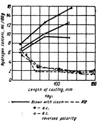
Fig. 78. Variations in hydrogen content in ingots of steel X25H2O cast by electric slag process with d. c. and a. c.
