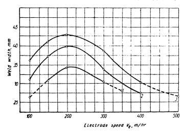
Fig. 24. Weld width vs. speed of wire feed on various thicknesses of metal per electrode  $\frac{\delta}{n}$ :
