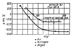
Fig. 60. Effect of gas shielding on manganese content in ingot (CB-151 wire and AH-8 flux).
