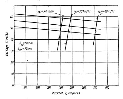
Fig. 20. Welding current vs. welding voltage in electric slag welding with a constant-voltage transformer.
