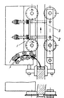
Fig. 145. Diagram of a trackless welding unit.
