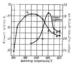
Fig. 211. Effect of quenching temperature on hardness and impact toughness of X12BP deposited metal (tempering at 200° for 1.5 hours).
