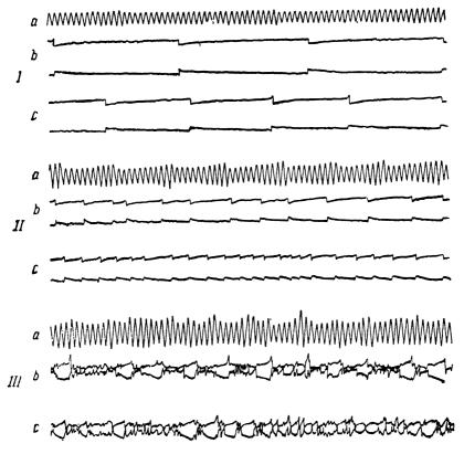
Fig. 75. Wave forms of electric slag welding with a. c. and d. c.:
