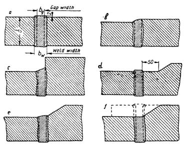
Fig. 81. Types of butt joints.
