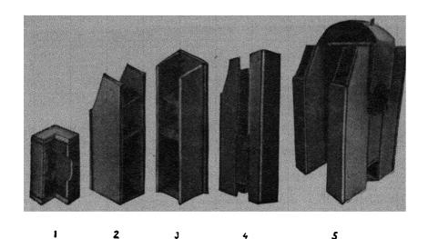
Fig. 249. Parts of the frame of a 4,000 ton forging press:
