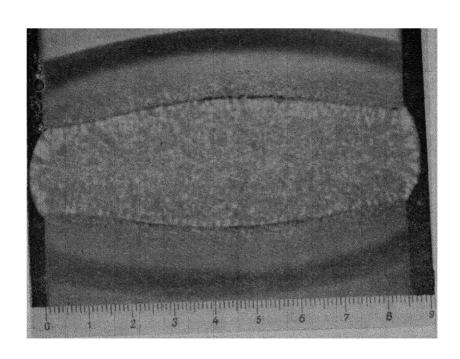
Fig. 195. Tears in near weld zone at line of fusion in electric stag welding.
