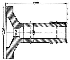
Fig. 252. Shaft for a hydraulic turbine.
