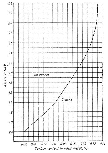
Fig. 189. Carbon content in welds plotted as a function of aspect ratio at which no crystallisation cracks occur. 0.7-1.5 per cent Mn; 0.35 per cent Si; Mn/Si≥18.
