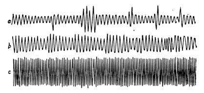
Fig. 72. Current oscillograms in electric slag welding a—drop transfer at welding voltage of 31-32 v; b—ditto, at 44-46 v; c—ditto, at 55-56 v.
