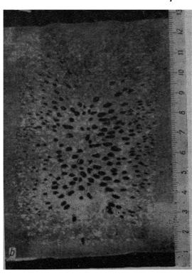
Fig. 76 Gas pockets in electric slag weld:
