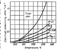
Fig. 80. Variations in electrical conductivity of existing flux grades with tem-
