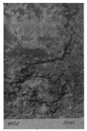
Fig. 117 Crack extending from the near weld zone into the weld metal (×8).
