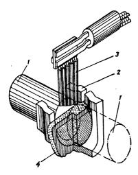
Fig. 255. Multielectrode welding of reinforcing bars with slag run off:
