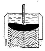
Fig. 41. Schematic diagram of metal pool in welding with one fixed electrode.
