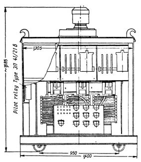
Fig. 168. Type TIIIC-1000-3 three-phase transformer for electric slag welding.
