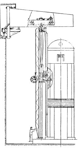
Fig. 161. Crane-type universal unit incorporating an A-372 welding apparatus.
