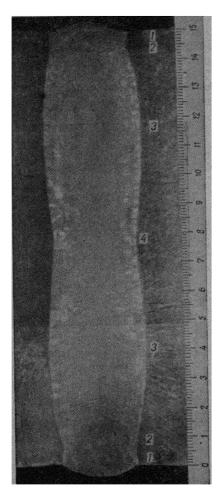
Fig. 38. Electric slag weld made with one weaving electrode.
