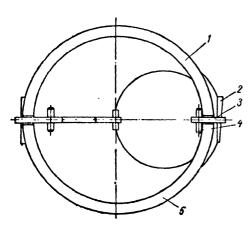
Fig 225. Diagram showing a shell fitted up for welding by means of spacers and wedges:
