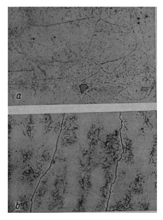
$a = alloy \ \partial W435$  (magnification  $\times 300$ ),  $b = electric slag weld (magnification <math>\times 150$ ).
