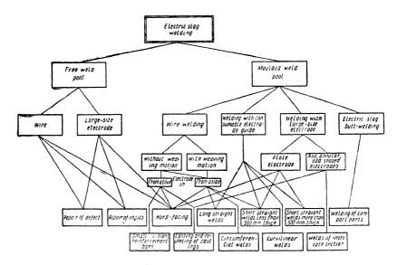
Fig. 6. Electric slag welding classification.
