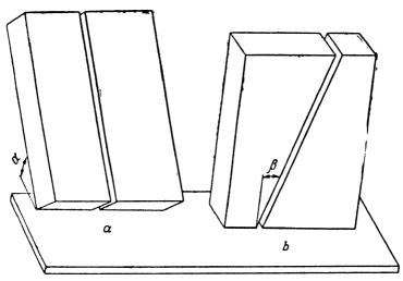
Fig. 85. Tilt of weld in the electric slag process.
