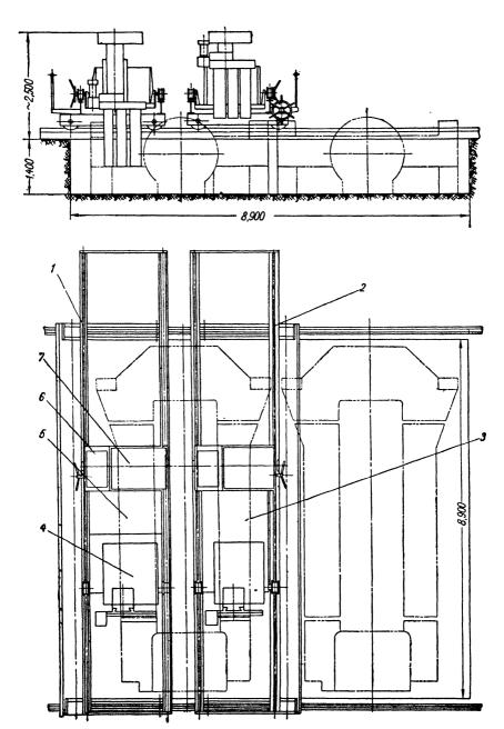
Fig. 163. Welding unit for rectangular heavy sections; 1, 2-jibs; 3, 5-trucks; 4-A-480 welding apparatus; 6-control cabinet; 7-transformer.
