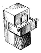
Fig. 100. Diagram of hard-facing of a flat surface in a vertical position by means of composite moulding shoes.
