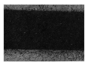
Fig. 205. Poor lusion in electric slag welding.  $a = \text{steel } \partial M654$ ;  $b = \text{alloy } \partial M437B$ ,  $c = \text{steel } 1 \times 18 \text{ H9T}$ (magnification  $\times 150$ ).
