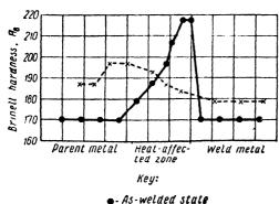
Fig. 183. Brinellhardness of welded joints before and after normalising.
