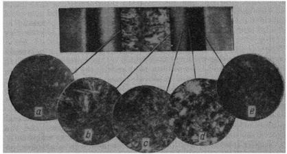
Fig. 193. Microstructure and hardness of 30X2H3MA Cr-Ni-Mo steel in near-weld zone after electric slag welding (magnification ×300).
