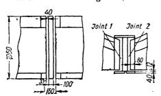
Fig. 109. Bedplate prepared for welding.
