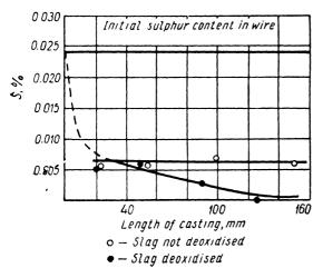
Fig. 69. Sulphur content variations in deposited metal in electric slag welding with flux containing 70 per cent CaF<sub>2</sub> and 30 per cent CaO, with and without deoxidation of slag pool surface.
