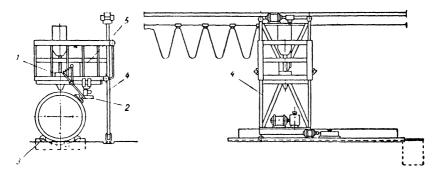
Fig. 164. Welding unit for boiler drums.
