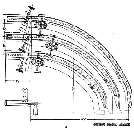
Fig. 142. Electrode guides and moulding shoes
