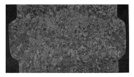
Fig. 209. Macrosection taken across butt weld made by the electric slag process in commercial titanium.
