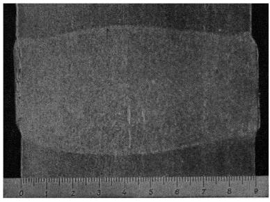
Fig. 200. Macrograph of a welded joint in Cr-Ni-Mo steel after hardening and tempering.
