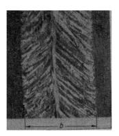
Fig. 21. Weld width in electric slag welding.
