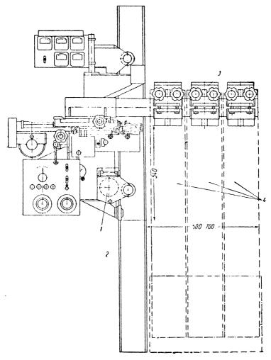
Fig. 139. Type A-372P welding apparatus using plate electrodes:
