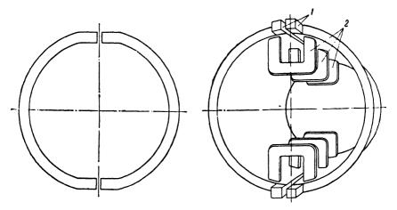
Fig. 220. Shell course formed on rolls in preparation for welding.
