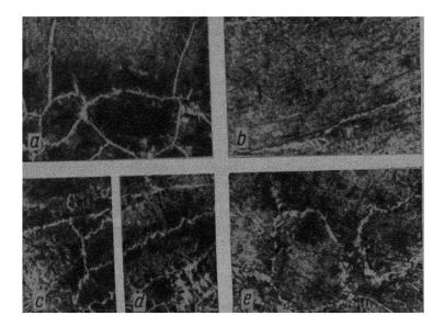
Fig. 54. Secondary structure of weld metal (magnification $\times$ 60):
