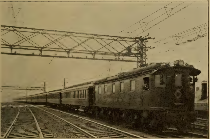
FIG. 140.—NEW YORK, NEW HAVEN & HARTFORD GEARED LOCOMOTIVE. Number 071 hauling the 12-coach "Boston Express."
