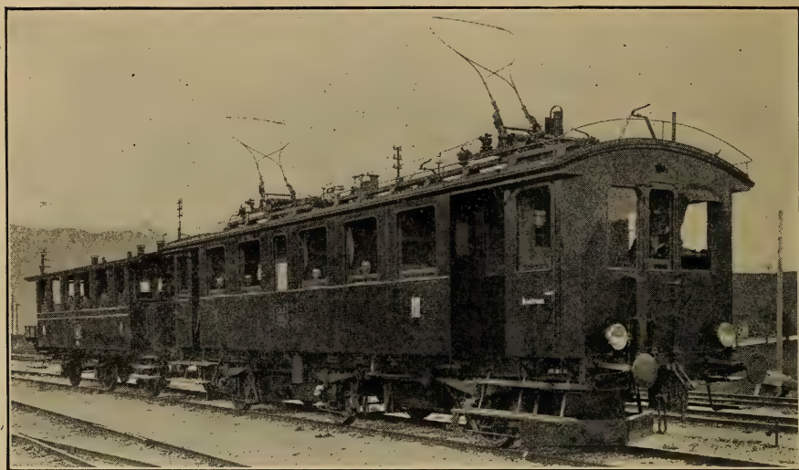
FIG. 81.—BAVARIAN STATE RAILWAY. MURNAU-OBERRAMMERGAU LINE MOTOR CAR TRAIN. Two 100-h. p., single-phase Siemens motors per motor car and coach.
