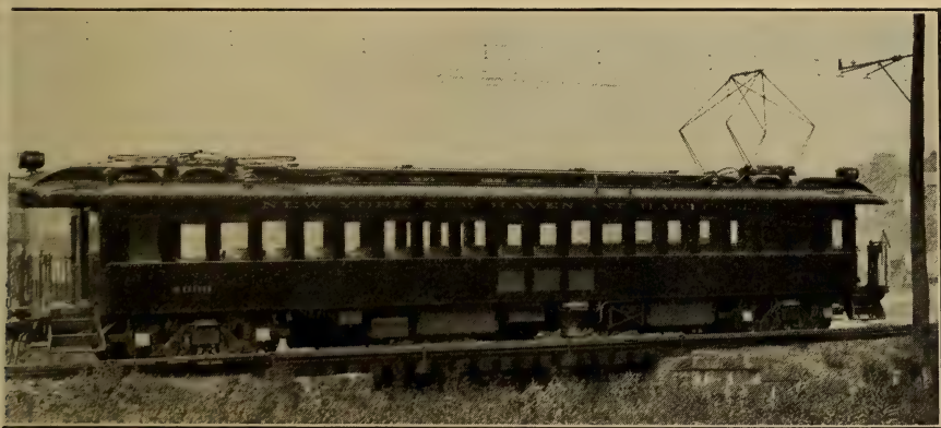
FIG. 71.—NEW YORK, NEW HAVEN AND HARTFORD MULTIPLE UNIT 87-TON MOTOR CAR. Operated in trains on the New York Division, 1909.
