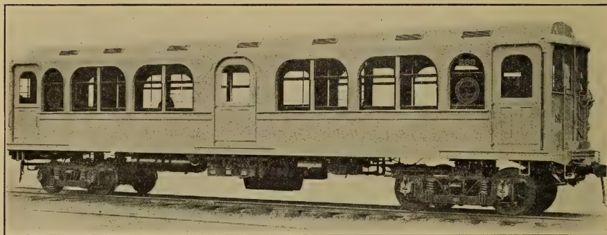
FIG. 54.—HUDSON AND MANHATTEN RAILROAD MOTOR CAR. Length 48 feet; seats 44; weight 35 tons; builder, Pressed Steel Car Company.
