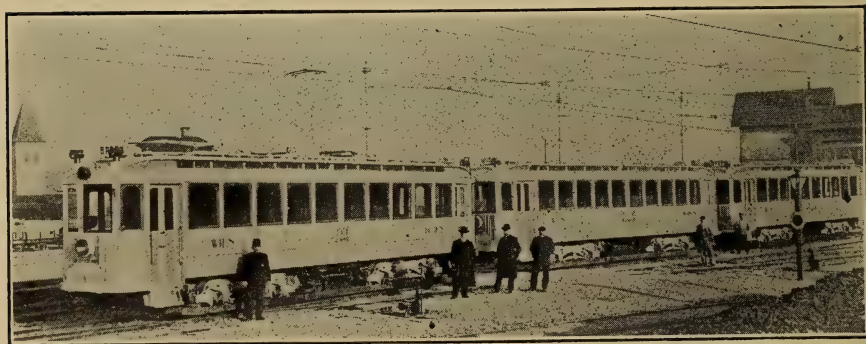
FIG. 82.—VIENNA-BADEN RAILWAY. MOTOR-CAR TRAIN. Four 60-h. p., single-phase motors per motor car.
