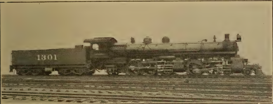
FIG. 24.—ATCHISON, TOPEKA & SANTA FE. MALLET ARTICULATED LOCOMOTIVE. Cylinders 24 and 38 by 28; heating surface 4756 square feet; weight 610,000 pounds, with 12,000 gallons of water and 4000 gallons of oil.
