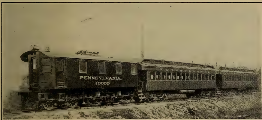
FIG. 129.—PENNSYLVANIA RAILROAD. EXPERIMENTAL LOCOMOTIVE AND TRAIN, 1909. Single-phase gearless motors.
