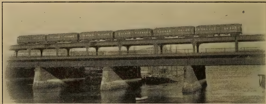
FIG. 52.—BOSTON ELEVATED RAILWAY MOTOR-CAR TRAIN. Car body length, 60 feet. Seating capacity, 64 passengers. Weight, 54 tons.
