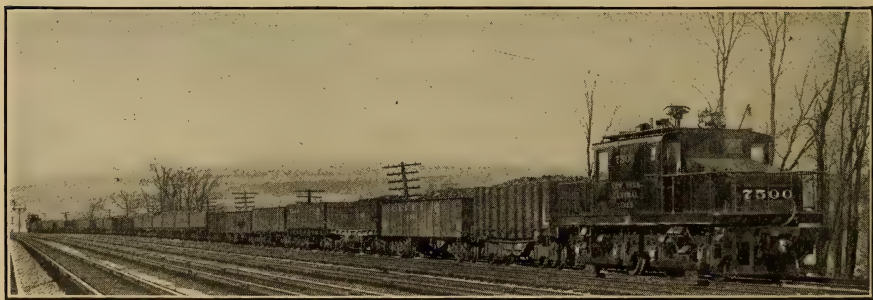
FIG. 100.—MICHIGAN CENTRAL RAILROAD. ELECTRIC LOCOMOTIVE AT DETROIT RIVER TUNNEL HAULING 1400-TON FREIGHT TRAIN.
