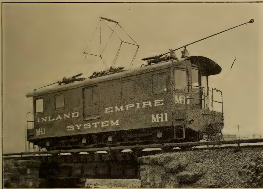
FIG. 132.—SPOKANE AND INLAND EMPIRE RAILROAD FREIGHT LOCOMOTIVE, 1910. One of eight, 72-ton, 680-h. p., geared, single-phase units.
