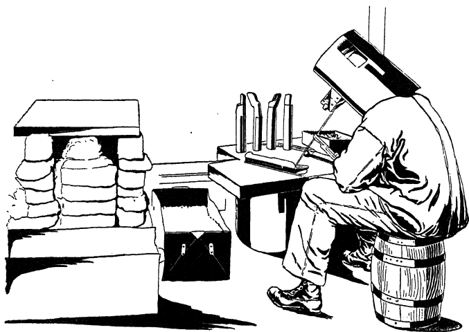
FIG. 147.—Welding High-Speed Tips Onto Mild Steel Shanks.
