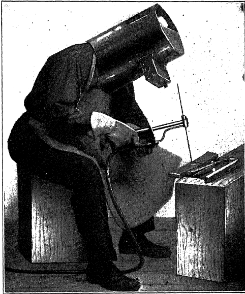
FIG. 36.—Correct Welding Posture and Equipment.
