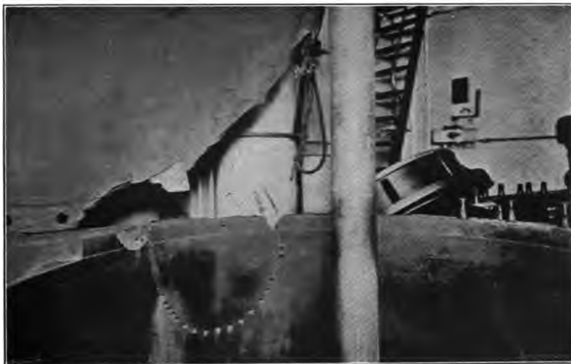
FIG. 74.—S.S. Prinz Joachim —Broken Cylinder-Head and broken Low-Pressure Cylinder.
