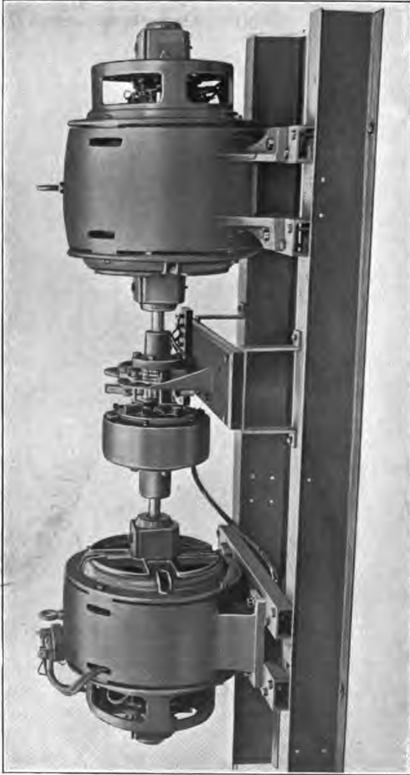
FIG. 41.—The Davies-Soames Clutch connecting a Motor to a Generator.
