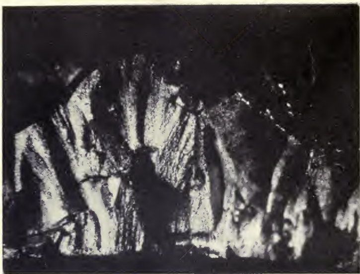
FIG. 1.—Fractured Surface of an Iron Deposit. \times 80 .
