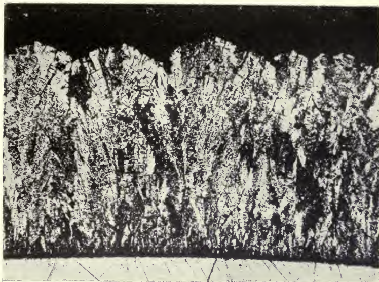
Dentate periphery—crystalline macroscopically.
