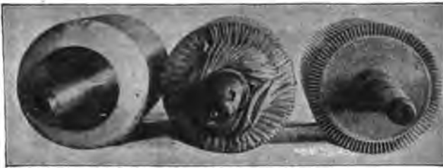
FIG. 18.—A TOOTHED-CORE ARMATURE SHOWING THE STAGES OF WINDING.
