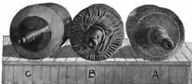
FIG. 130.—TOOTHED-CORE ARMATURE IN VARIOUS STAGES OF CONSTRUCTION.
