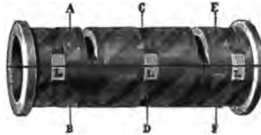
FIG. 144.—SLEEVE OF BABBITT METAL IN JOURNAL BEARING.
