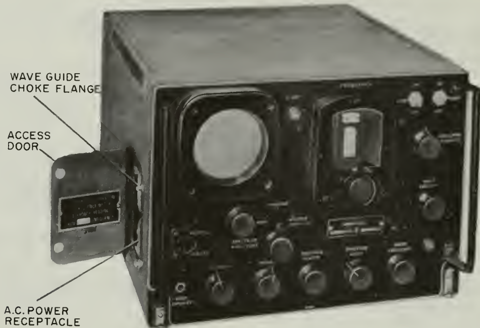
Figure 3-12.—Spectrum analyzer control panel.
