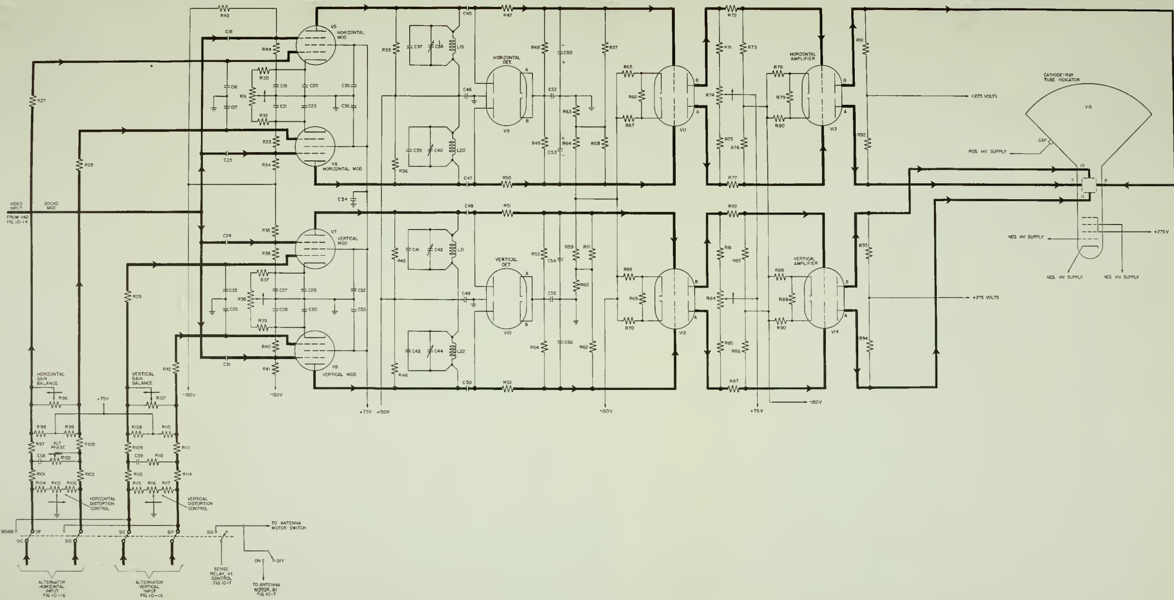
Figure 10-15.—Azimuth indicator (horizontal and vertical modulators and amplifiers).
