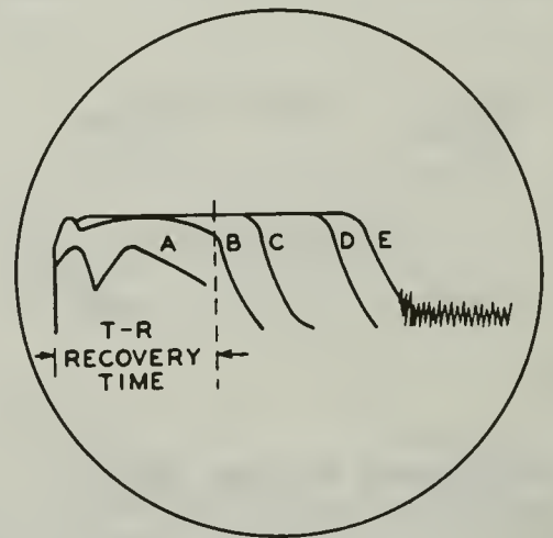
Figure 3-33.—Checking T-R box recovery.
