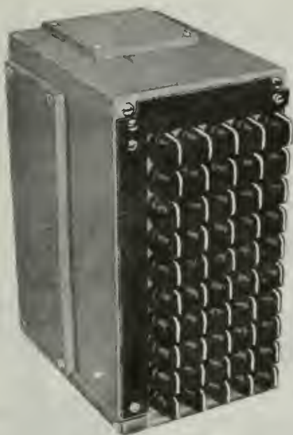
Figure 7-22.—External view of the Receiver Switchboard type SB-82/SRR.
