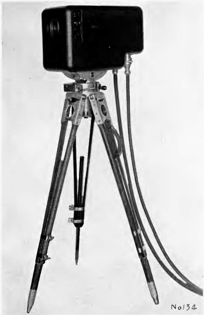
Fig. 13. The Farnsworth Pick-Up Camera complete. (Note compactness)
