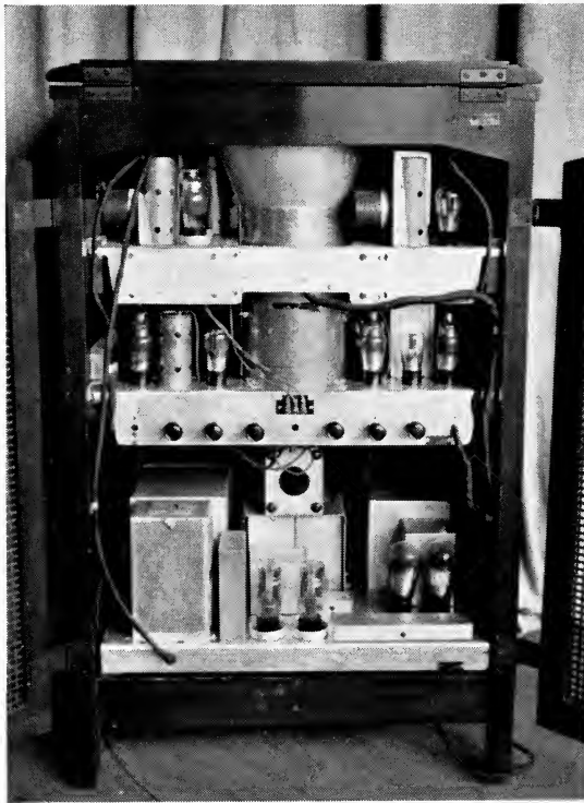
Fig. 65. Rear View of R.C.A. Receiver. Note the Kinescope placed vertically
