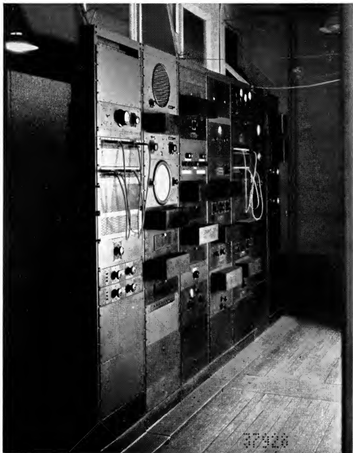
Fig. 22. The Control Panel of the R.C.A. Experimental Television Station in Camden, New Jersey
