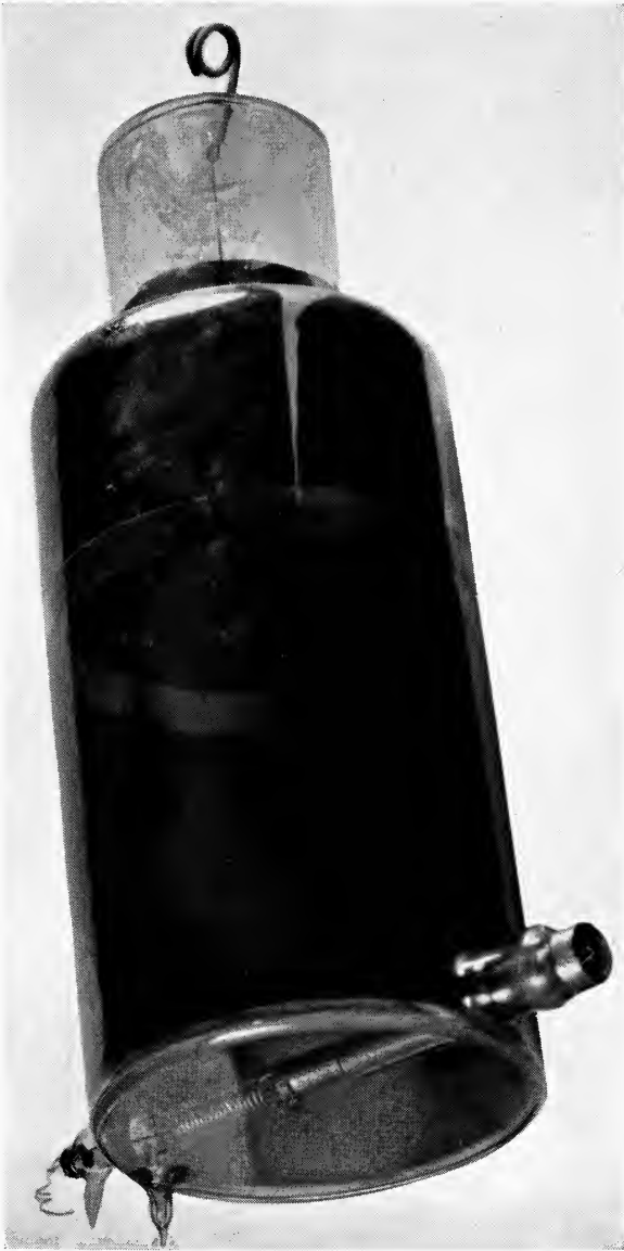
Fig. 12. Farnsworth Image Dissector Tube with Multiplier
