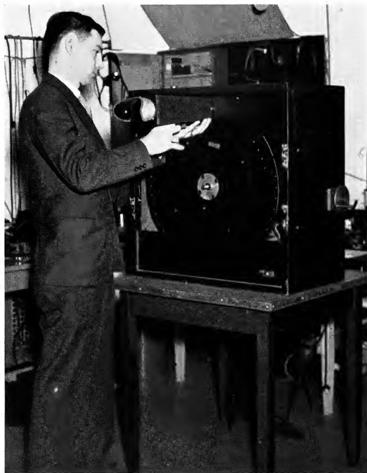
Fig. 33. Mechanical Scanning Television Receiver. The large disk is driven by a high-speed motor
