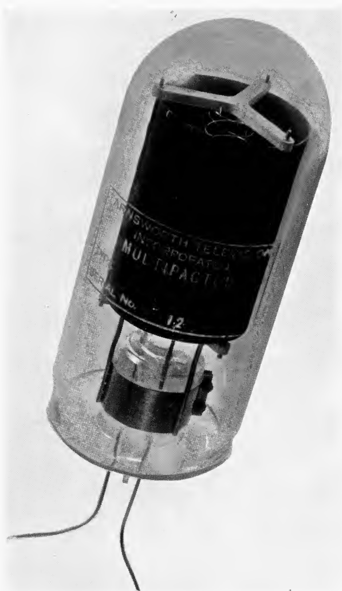
Fig. 69. Farnsworth Multipactor Tube
