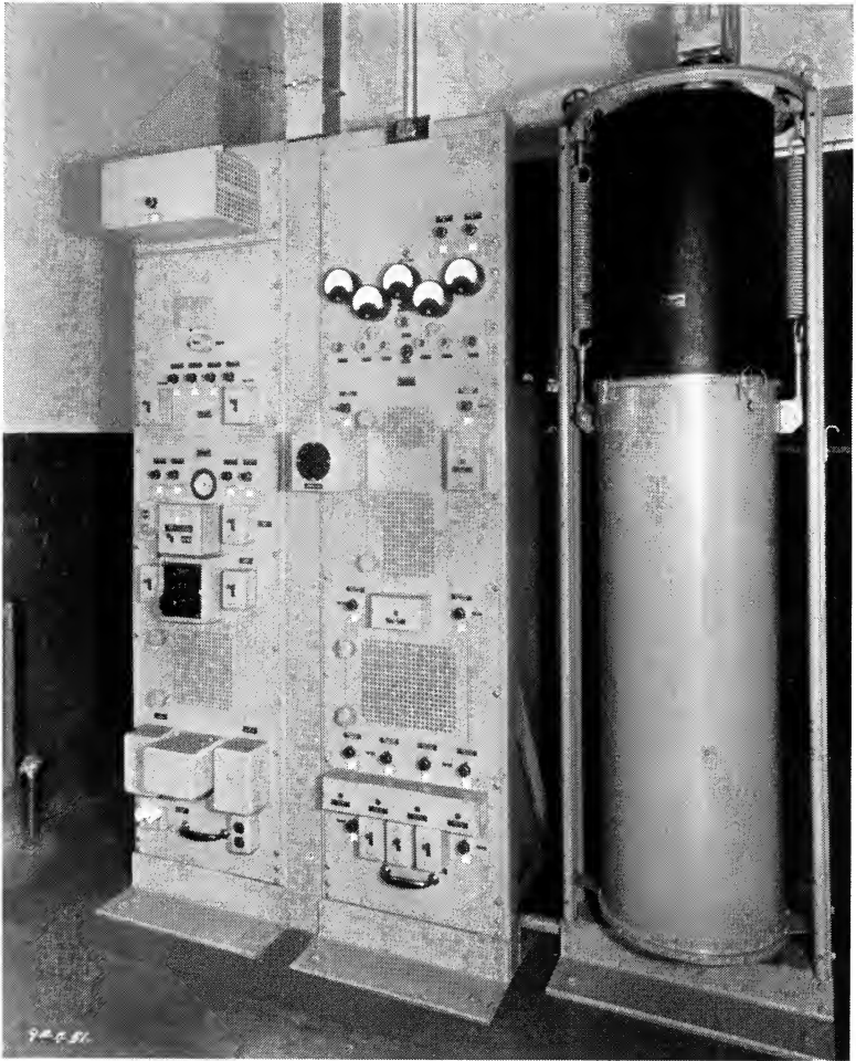
Fig. 81. Three Meter Transmitter Used in R.C.A.'s New Ultra-Short Wave Radio Circuit Connecting New York and Philadelphia
