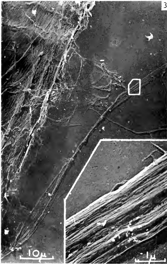
Fig. 3. Carbon replica, metal-shadowed, of a beaten spruce tracheid and its associated fibrillation. Magnification 1500, inset 13,000.
