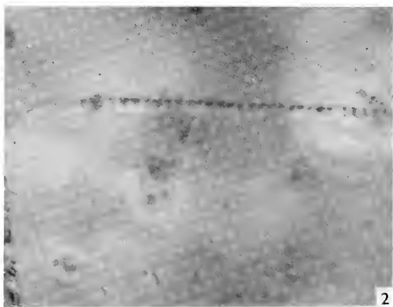
Fig. 2. A sub-boundary consisting of uniformly spaced dislocations. The average spacing of the dislocations is about 175 Å. Magnification 120,000.
