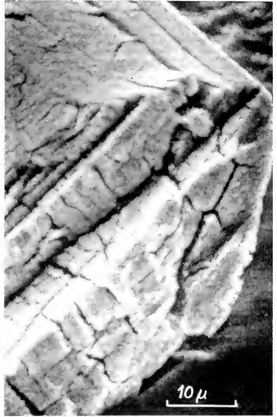
Fig. 2 b. End of needle crystal of lead styphnate. Note crystallographic break-up due to dehydration.
