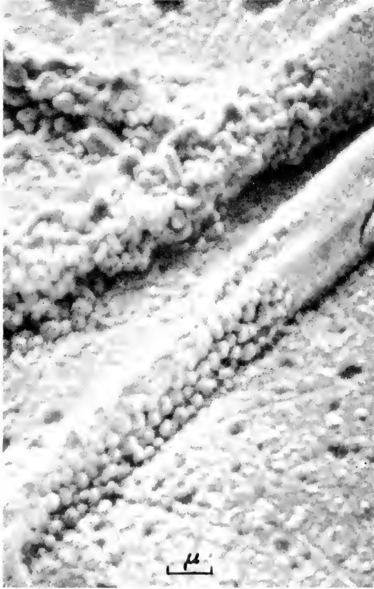
Fig. 2 a. Needle crystal of silver azide—partly decomposed by heat.
