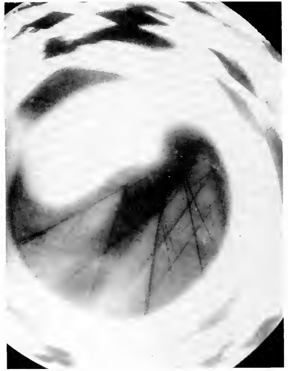
Fig. 4. Kikuchi lines of MgO crystals obtained in the caustic of a strong permanent magnetic lens.
