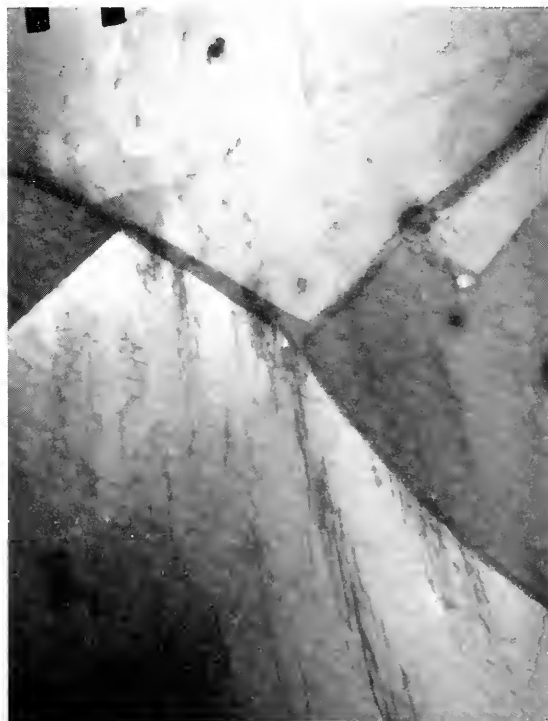
Fig. 2. Network of dislocation lines in lightly rolled steel.
