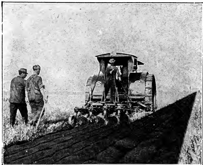
FIG. 58. A tractor engine drawing four plows.
