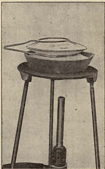
FIG. 20. Sand bath, filter paper, and double watch glass arranged to sublime benzoic acid
