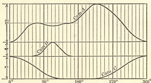
FIG. 17.—TIME CHART DIAGRAM, BASE CURVES SEPARATED
