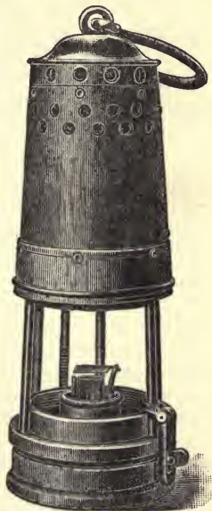
FIG. 76. Miner's lamp fitted with the Cunynghame-Cadman device.
