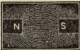
FIG. 73. — Field due to Opposite Poles.
