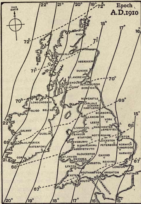
MAGNETIC CHART OF THE BRITISH ISLANDS SHOWING THE LINES OF EQUAL MAGNETIC DECLINATION AND THOSE OF EQUAL MAGNETIC DIP
