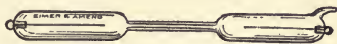
FIG. 35. — A form of tube in which gases are electrically heated to incandescence.
