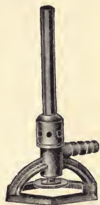
FIG. 2.—Tirrill burner. A modification of the Bunsen burner suitable for gasoline gas, as well as for coal gas.
