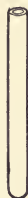
FIG. 6. — Glass tube closed at one end. The narrow thread of glass (Fig. 5) is melted and drawn off. The end of the tube is then softened in the flame, and, by blowing, either rounded off or expanded into the bulb of a matrass (Fig. 7).
