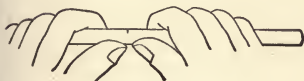
FIG. 3.—Breaking a piece of glass tubing. Make a scratch on one side of the tubing with a single stroke of the file. Place the thumbs on the other side of the tubing, directly opposite the file mark. Grasp the tubing with the thumbs and press backwards towards the thumbs.
