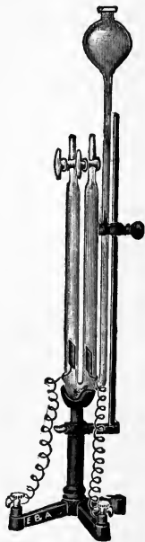
FIG. 18.—Hofmann's apparatus for the electrolysis of water.
