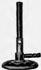
FIG. 1. — Bunsen burner . Ordinary form for use with coal gas.
