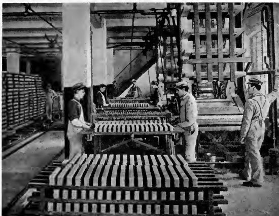
Cutting Soap Slabs into Bars
