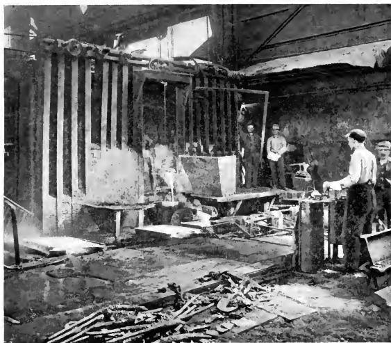
Casting Copper in Anode Molds
