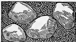
Sand Filling Voids between Large Stone (poor)
