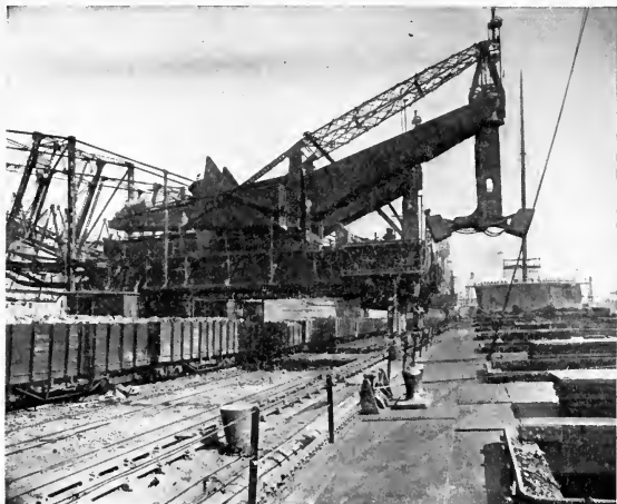
Derrick Unloading Ore from a Boat at a Wharf
