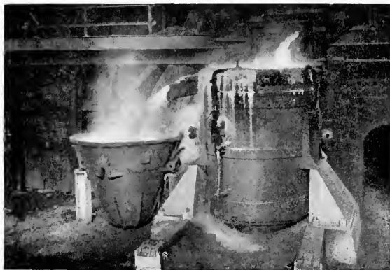
Molten steel is shown flowing from the open hearth furnace into a ladle. The smaller thimble-shaped vessel receives the slag which rises to the top and flows over into it.
