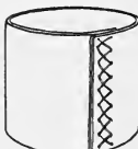
bring two ends of strip together lapping 1/2" sewed together forming a hollow cylinder
