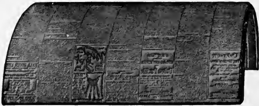
A Stereotype Plate Curved to Fit the Press Cylinder
