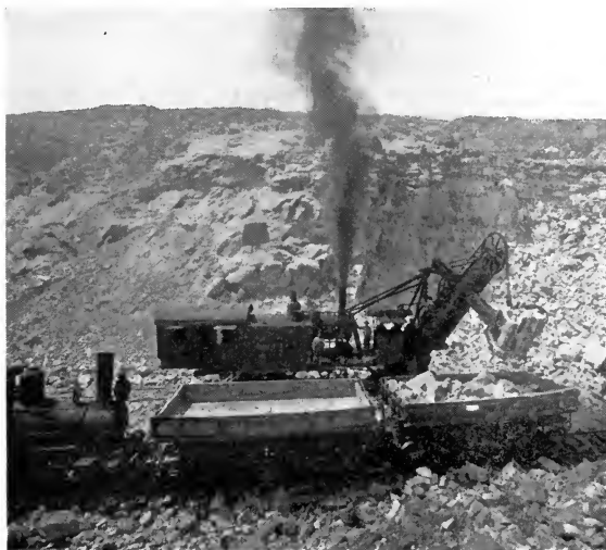
Courtesy of New York and New England Cement & Lime Co. Steam Shovel in Operation in Limestone Quarry
