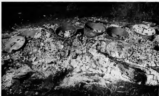
KETTLES AFTER THE FIRE HAS DIED DOWN The covers have been removed to show the fired ware
