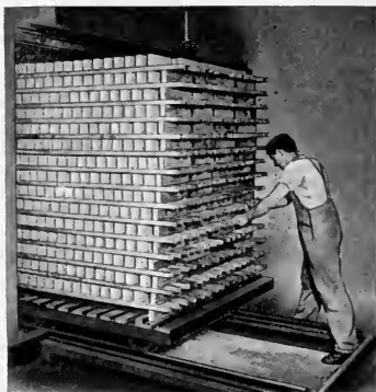
Soap on Racks Going into Dryer
