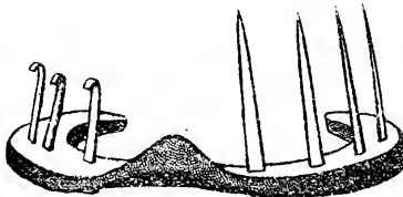
2. Shoe and Nails, in situ , showing the inward direction of the Nails when driven into the Hoof. Right Side of Shoe showing Clinches turned over.
