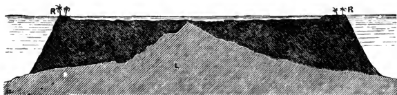
FIG. 41.—Section of an Atoll or coral island (R R) built over submerged land (L).
