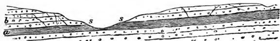
FIG. 43.—Section across a valley to show how the simplest kinds of springs arise.
