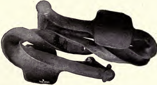
FIG. 89.—A High-Grade Drop Forging Bent and Twisted Cold.
