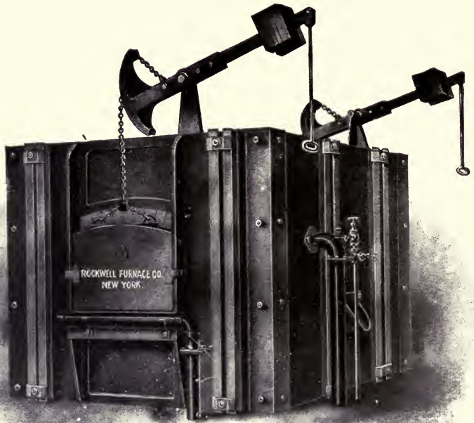
FIG. 50.—Furnace for Reheating Billets.
