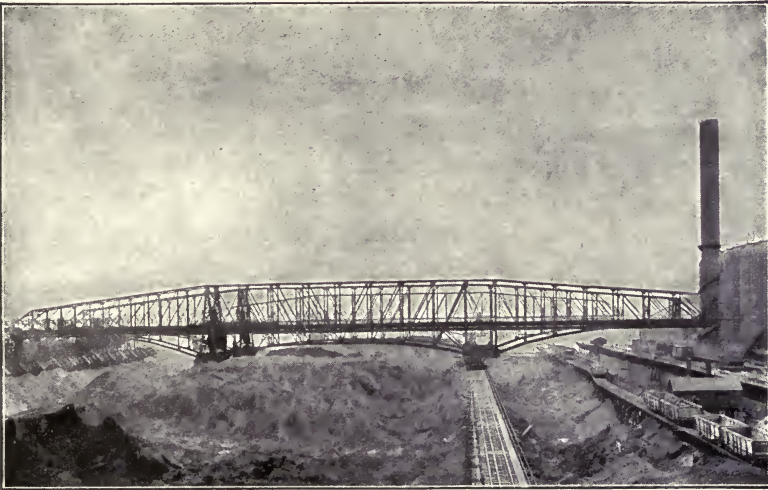
FIG. 15.—Bridge crane for handling ore. The unloading hoists on the left take ore from vessels lying under them and pass it to the bridge crane in transfer cars. This crane carries it to its proper pile, according to composition, and also carries ore to the charging cars of the furnaces on the right.
