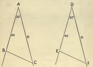
Adjust the bevel, or protractor, to the angle **B**, and also to the angle **E**, and carefully compare the magnitudes of these two angles. In like manner compare the magnitudes of the angles **C** and **F**. With the dividers compare the magnitudes of the sides **BC** and **EF**.
