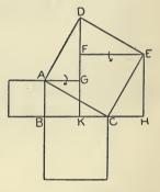
equal to the triangle ABC; and cutting out the triangle AGD, it may be turned about A, in the direction indicated by the arrow head, into the position ABC. Measurement will also show that the triangle EFD is in all respects equal to the triangle EHC; and cutting out the triangle EFD, it may be turned about E, in the direction indicated by the arrow head, into the position EHC. We thus have the square on AC converted into ABKG and FKHE, which will be found to be the squares on AB and BC.
