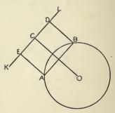
The chord AB is equal to ED, and therefore is of the required length, and it is parallel to KL.
