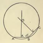
with which the angle ABC (135°) is constructed, AB and BC are bisected, and the perpendiculars KO and LO are drawn.
