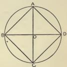
Of course the evident equality of the triangles AOB, BOC, . . . proves the equality of the sides, and the angles ABC, BCD ... are all right angles, because they are angles in semicircles.
