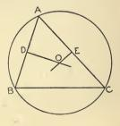
perpendicular to **AB** and **AC**, respectively. Then all points in **DO** are equally distant from **A** and **B**; and all points in **EO** are equally distant from **A** and **C**. Hence **O** is equally distant from **A**, **B** and **C**; and if the sharp point of the compasses be placed at **O**, and the pencil end at **A**, or **B**, or **C**, and a circle be described, it will pass through **A**, **B** and **C**.
