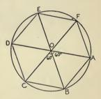
the three sides of these angles both ways to the circumference, and join the succeeding points of intersection. The construction being accurately made, the bevel will show the equality of the angles ABC, BCD, ..., and the dividers will show the equality of the sides AB, BC, .....
