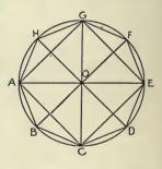
square in the circle. Through the centre, using parallel rulers, draw diameters parallel to the sides of the square. The quadrants are thus bisected, and we get eight equal angles at the centre. Joining ends of the successive radii which bound these angles, we have an octagon inscribed in the circle. The accuracy
