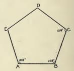
Joining E and D, we have a regular pentagon ABCDE. Using the bevel, we shall find that the angles at E and D are equal to the three other angles, and the dividers will prove the side DE to be equal to the other sides.
