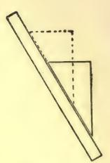
right angle of set-square against the latter, we are often unable to bring the perpendicular up to the line by reason of the right angle of the set-square having become rounded through use.
