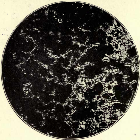
FIG. 63.—1·2 per cent. Carbon Steel (quenched from 700° C.). × 150.
