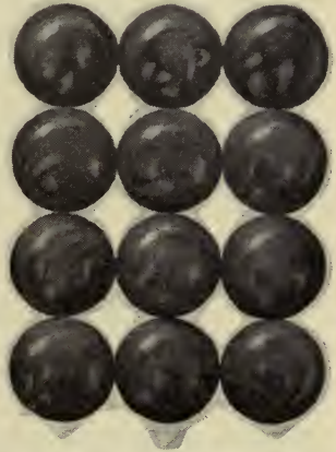
Fig. 39. Diagram to illustrate how the soil particles are covered by capillary water.
