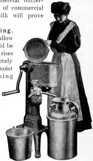
Fig. 163. A modern cream separator.
