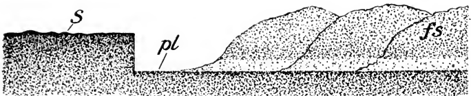
Fig. 40. Diagram to illustrate the effect of ideal plowing. The compactness of the soil is indicated by the density of the shading. Before plowing, there is a compact surface crust ( s ), below which the soil grows less compact as we go deeper; after plowing, this compact mass is broken up into a loose, friable mass of soil-crums, or floccules, with a consequent increase in the bulk of the furrow-slice ( fs ); compacted plow sole at pl . Modified after Hilgard.
