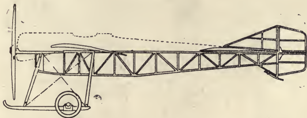
FIG. 48.—RIGID TYPE OF GIRDER FUSELAGE.
