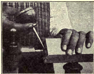
Fig. 7. Oiling the Dead-center.
