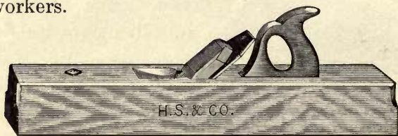
FIG. 28. The Wooden Plane
