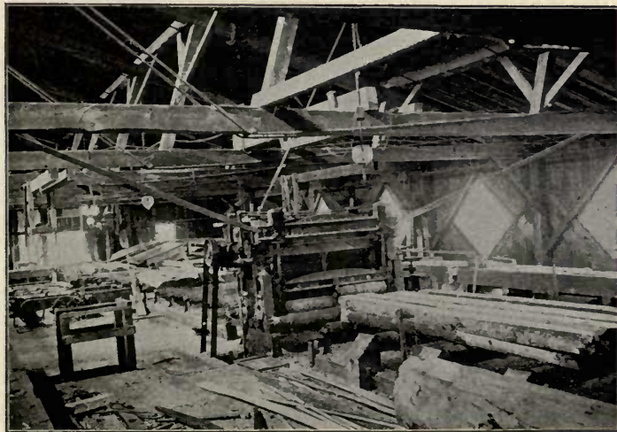
FIG. 68. A Modern Gang Saw — Interior of Modern Sawmill
