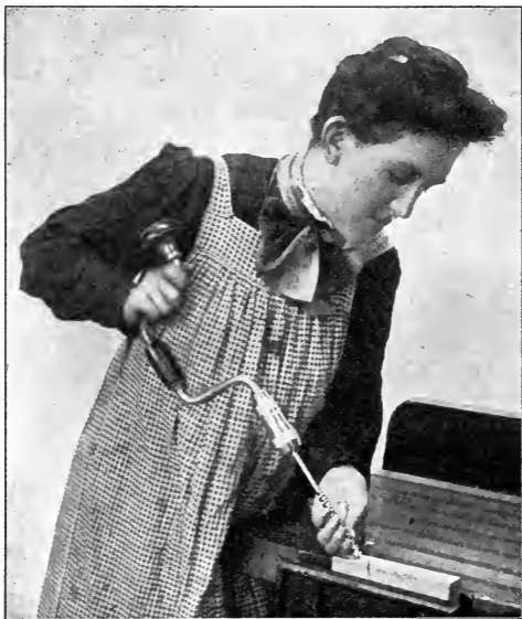
Fig. 71. Setting a Bit to Bore a Hole.
