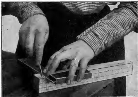
Fig. 42. Lining Around an End. Compare the position of the try-square and fingers shown in this figure with the positions shown in Figs. 19, 20, 21, 32, and 33.
