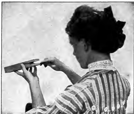
Fig. 75. Testing the Sides of the Mortise with a Narrow Chisel.
