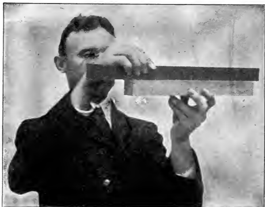
Fig. 5. Using a Straight Edge. Learn to examine the edge as shown in Fig. 2. The straight edge should be used only to see whether the first test has been successful.
