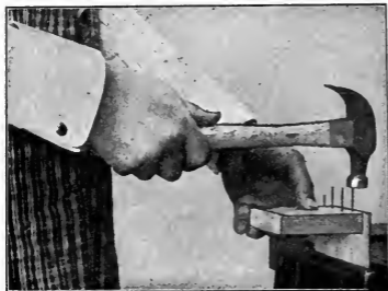
Fig. 108. Nailing a Rabbeted Corner.
