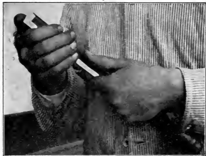
Fig. 165. Testing an Edge with the Thumb.
