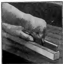
Fig. 18. Marking off Spaces.
