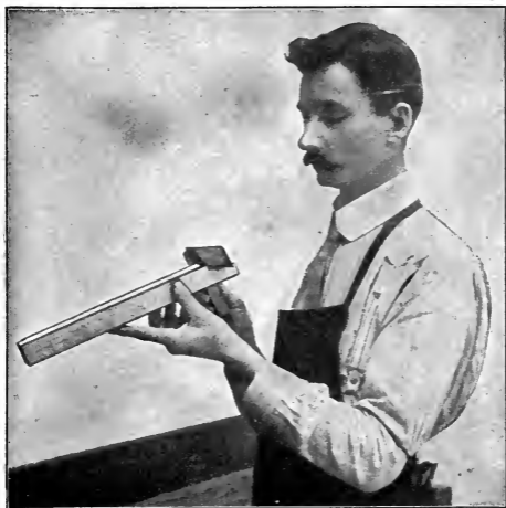
Fig. 55. Testing a Grain with a Try-Square. The head of the try-square is not held against the piece.
