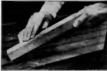
Fig. 46. Sandpapering a Side. Compare this view with Fig. 47.
