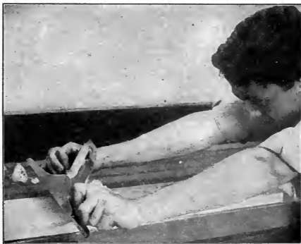
Fig. 96. A Plane Used as a Straight Edge.
