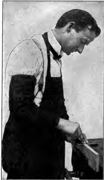
Fig. 32. Lining on an Edge. Notice that the workman stands erect with the hands in an easy position. Compare the position of the try-square with that shown in Fig. 33.
