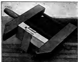
Fig. 77. First Clamp on the Slip Mortise and Tenon.
