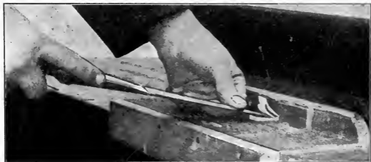
Fig. 83. Making a Wedge.
