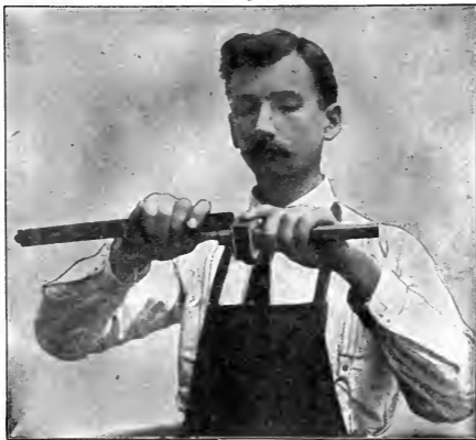
Fig. 14. Setting the Gauge.
