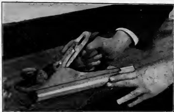
Fig. 125. Planing an Octagon Against a Bench-Stop.
