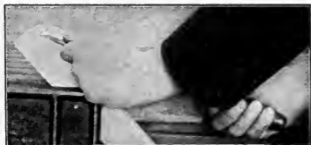
Fig. 106. Chiseling a Chamfer on a Circle.
