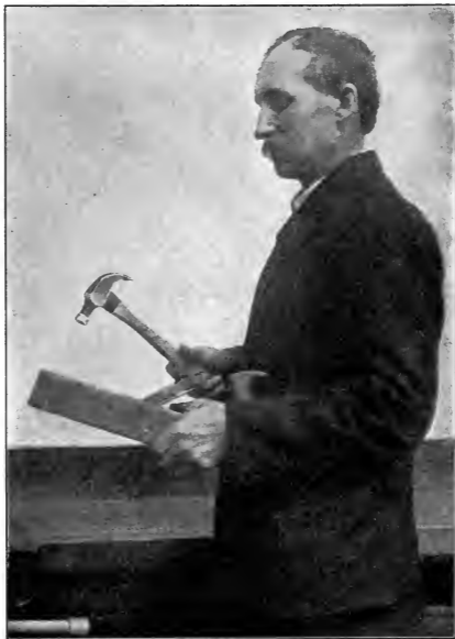
Fig. 171. Withdrawing the Plane Iron of the Wooden Plane.
