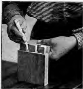
Fig. 92. Scribing in the Mortises for the Pins.
