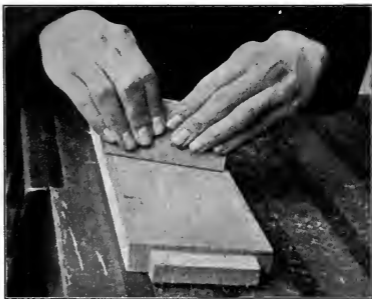
Fig. 191. Pulling a Scraper.
