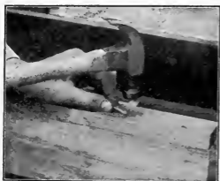
Fig. 28. Using a Nail for a Nailset.
