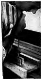
Fig. 76. Squaring the Inner End of the Mortise.
