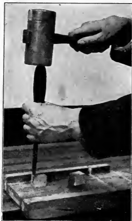
Fig 82. Splitting Material for a Wedge.
