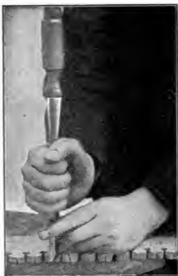
Fig. 40. Using a Chisel. Reverse Position.
