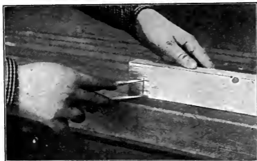
Fig. 105A. First Step in Locating the Point at Which to Set the Compasses.
