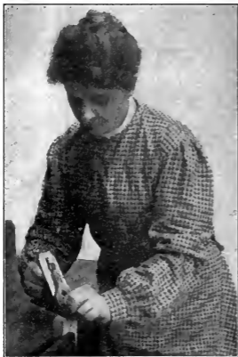
Fig. 98. Planing an End Square in the Vise.
