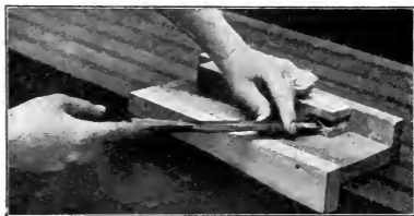
Fig. 73. Finishing the Sides of the Mortise. Compare this figure with the next one.
