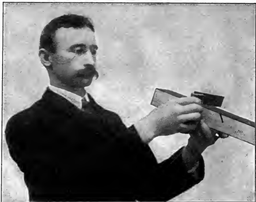
Fig. 12. A Try-Square on the First Edge. Observe carefully the position of the hands.
