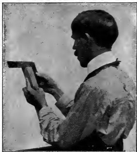
Fig. 56. Testing a Gain with a Try-Square. The head of the try-square is held against the face edge
