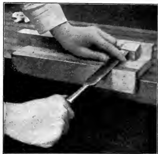
Fig. 53A. Chiseling at the Right Hand End.
