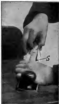
Fig. 173. Lifting the Cam Lever. S—The screw which holds the cap and iron in place.
