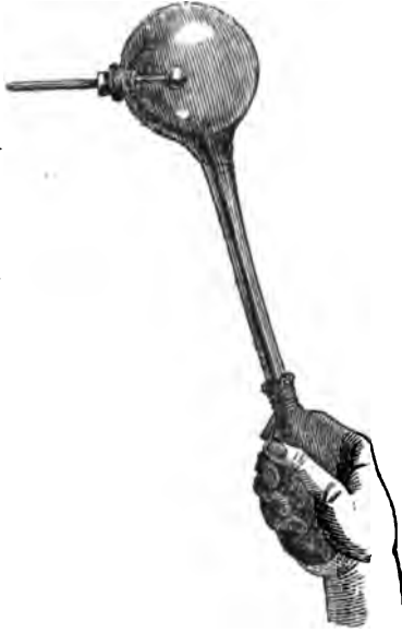
Apparatus for showing the influence of Relaxed Pressure, on the capacity of Air for Heat, or Moisture.
