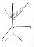
ses when at a greater distance from the origin, above or below, than the value of g in equation (3). Hence, the surface extends to infinity in all directions from the centre, and consists of two distinct and equal parts or nappes, as in the figure. It is therefore called, an Hyperboloid of two nappes.
