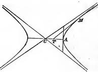
drawn to the hyperbola intersect the transverse axis between the centre and the vertex of that branch to which they are drawn; and the asymptotes are the limits of all tangents.
