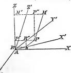
angles to each other, and AX', AY' and AZ', three oblique axes having the same origin. Denote the angles made by the new axis AX' with the three primitive axes of X, Y and Z, respectively, by X, Y and Z, those made by the axis AY'with the same, by X', Y' and Z',
