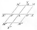
and AY; then if the distances MR and MP are given, it is evident that the position of the point M, will be known, and may be constructed, by laying off on the line AX, beginning at A, AP = RM, drawing PM parallel to AY; then on AY, laying off AR = PM and drawing RM parallel to AX; the point of intersection of these parallels will be the required point.
