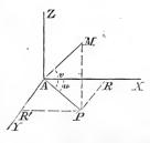
by referring them to any other three fixed objects. For instance, let A be a fixed point, and AX a fixed line in the given plane YAX, and let M be any point in space. If the distance AM, and the angles MAP and PAX are given, the position of the point is known, and may readily be constructed.
