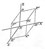
are given, it is evident that the position of the point will be fully determined, and may be constructed, thus: On AX lay off AR'' = MP''; on AY lay off AR' = MP'; through their extremities draw the lines R''P and R'P parallel respectively to AY and AX; through their point of intersection, P, draw PM parallel to AZ, and on it lay off the given distance, MP; the extremity will be the required point.
