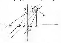
VV' in F, F is the focus through which the axis may be drawn parallel to DV.
