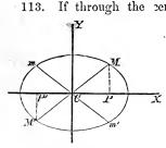
If through the centre of an ellipse any right line be drawn, its equation referred to the axes CX and CY, will be
