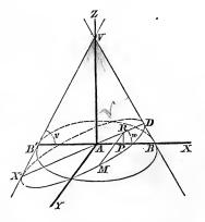
If the angle, made by the elements of the cone with the plane of the base, be denoted by v, we have in the right angled triangle VAB',
