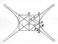
of all parallelograms described on the abscissas and ordinates of points of the curve, referred to the asymptotes, are equal, each being measured by the expression  $m \sin 2\alpha'$ .
