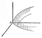
positive direction of the axis of X, but does not extend at all to the left of the origin; that the intersections by one system of planes are ellipses, and by the other two, parabolas. It is therefore called an *elliptical paraboloid*.
