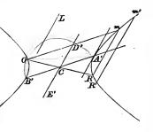
construct its conjugate. From the extremity of any diameter draw a chord Rm, parallel to the given diameter; draw the supplement, Om, of this chord; through the centre draw a diameter CA' parallel to this supplement, it will be
