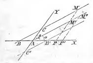
the co-ordinates AP and MP are denoted by x and y. Through the origin A, draw AM' parallel to BM. Represent the angle YAX by  $\beta$ , and MBX = M'AX by  $\alpha$ ; the angle PM'A = M'AY will then be represented by  $\beta - \alpha$ .
