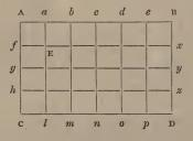
inches. Divide AB and CD (which are equal) each into 6 inches by the points a, b, c, l, m, &c.; and AC and BD (which are also equal) into 4 inches by the points f, g, h, x, y, and z. Join a and l, b and m,
