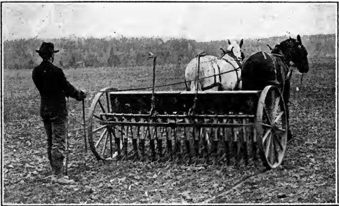
Figure 11.—Seeding with a drill. The dragging chains cover the seeds, which are placed in the ground at a uniform depth.
