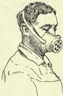
FIG. 24.—Form of respirator used by workers in certain dusty trades.
