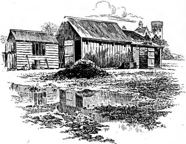
FIG. 34.—An Insanitary Cowshed and Dairy. Note the heap of manure and the collection of drainage close up to the entrance to the shed.
