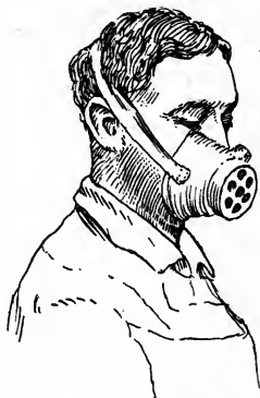
FIG. 24.—Form of respirator used by workers in certain dusty trades.
