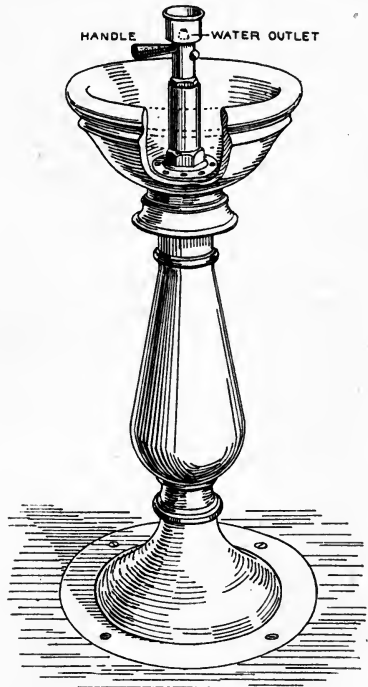
FIG. 98.—School Drinking Fountain. The water discharges upwards and the child drinks direct from the stream.
