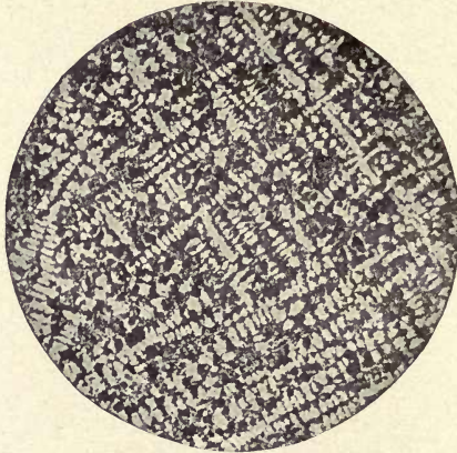
FIG. 38. 80% Au + 20% Sb, etched with NaOH. Magnified 27 times.
