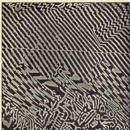
FIG. 22. 39% Sn, magnified 170 times.
