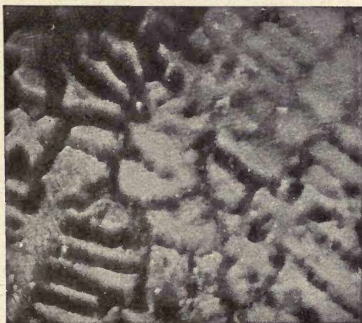
FIG. 62. 30% Cu + 70% Pd. Etched with dilute nitric acid and then re-polished. Magnified 70 times.
