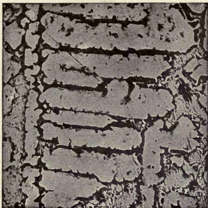
FIG. 25. 50% Sn, magnified 70 times.
