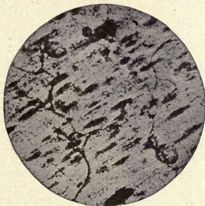
FIG. 65. 50% Iron + 50% Manganese (slowly cooled). Magnified 100 times.
