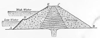
SECTION OF AN EARTHEN DAM.
