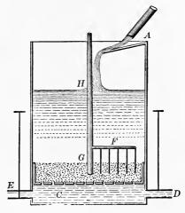
MECHANICAL GRAVITY FILTER.
