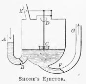
and opens F, and then the sewage is driven through the discharge pipe FG. As soon as the float falls to the level C its weight acts on the spindle so as to close the valve E; then the valve F falls by it own weight to prevent the sewage from returning to the ejector, and B is opened by the inflowing sewage.
