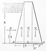
form is commonly used. The back of the dam where the water pressure is applied may be vertical or have a slight batter, but the front has always a considerable batter. The thickness of the top of the dam ranges from 4 feet for low heights up to 15 feet or more for heights of 100 feet. The batter of the back and the thickness of the top being assumed, the thickness of the base is to be computed so that there may
